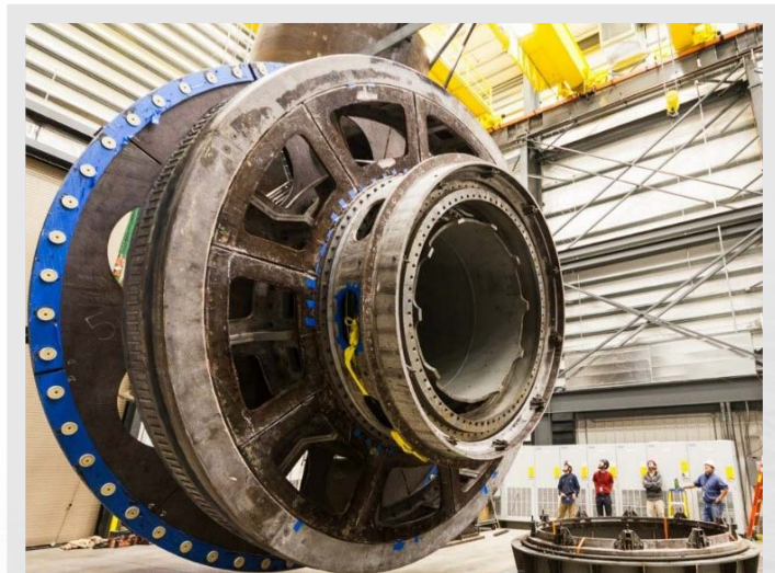
Figure 39. Columbia Power Technologies' wave energy converter is installed at NREL's 5-MW dynamometer at its Flatirons Campus.
