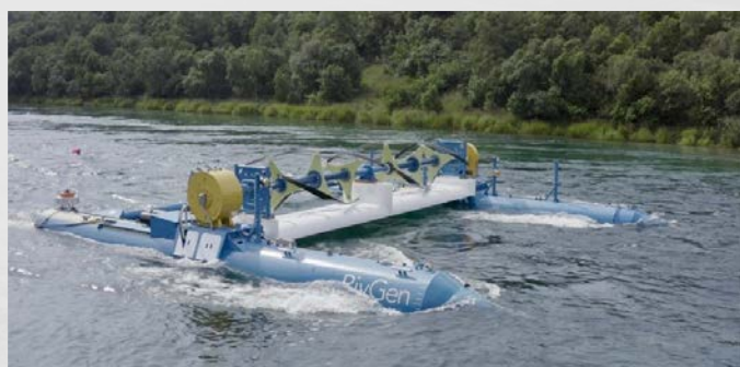
Figure 32. The ORPC RivGen Power System prior to installation on the Kvichak River in Igiugig, Alaska.
