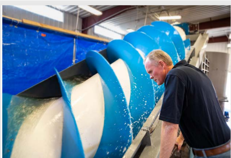
Figure 17. Percheron Power's composite Archimedes hydrodynamic screw.
