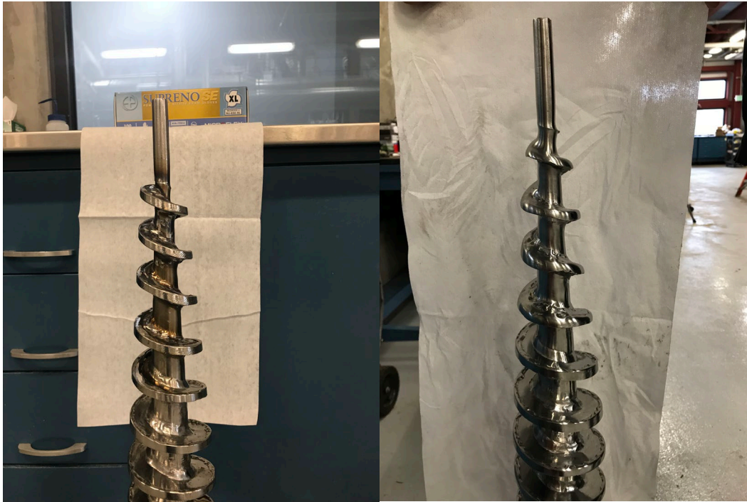
Figure 5. Wear on stainless steel 316 auger from corn stover (left: light wear; right: significant wear)
