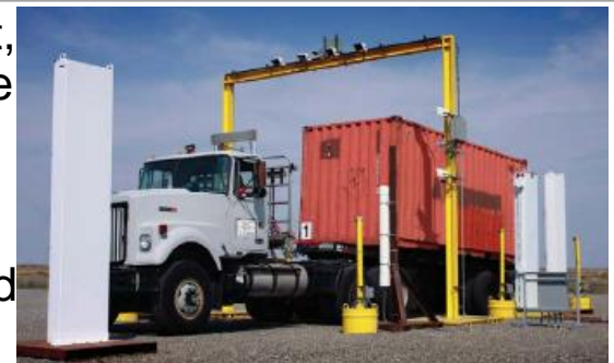
A container with naturally occurring radioactive processed through a radiation portal monitor as part of NNSA's Second Line of Defense Program.
