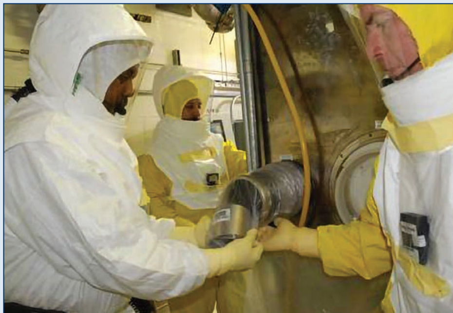
Employees at the SRS's K-Area resumed plutonium downblending after an outage for extensive upgrades on the KIS glovebox.
