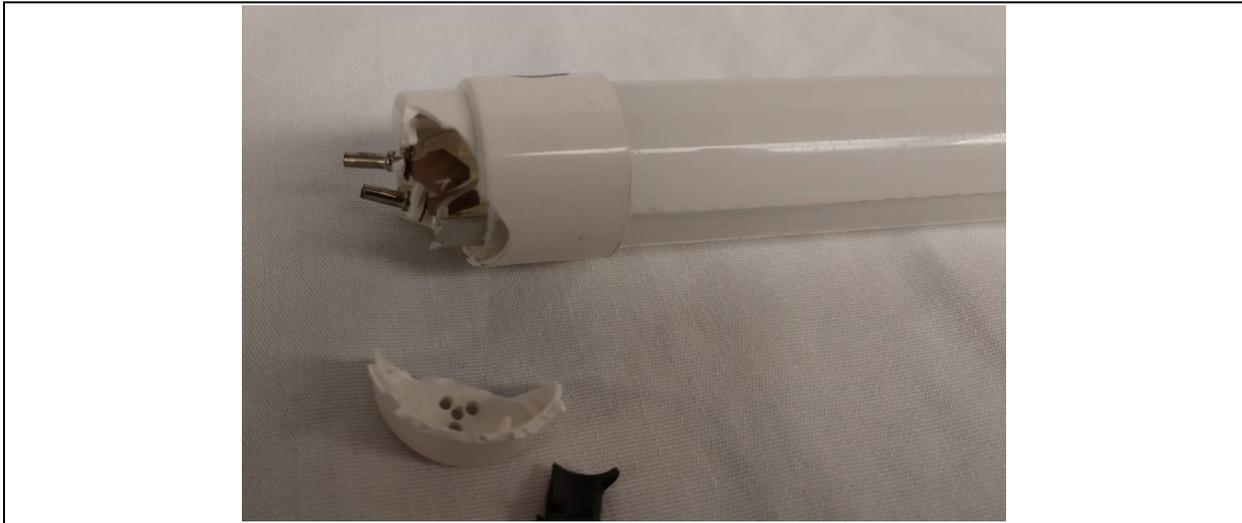
**Figure 3-4:** The base of a Product NB-1 DUT cracked and broke open during photometric testing after 7,000 hrs of 7575.
