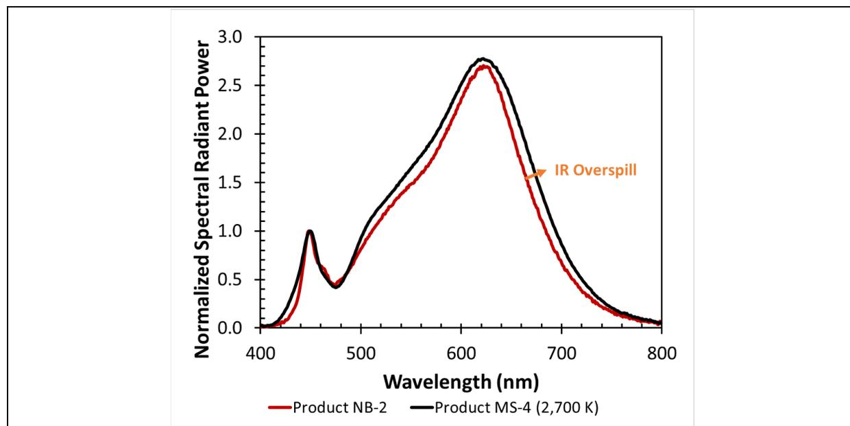
Figure 2-6: The SPD of Product NB-2 compared with a conventional all-phosphor reference (Product MS-4 at 2,700 K) shows reduced IR overspill. The SPD was normalized to blue emissions.
