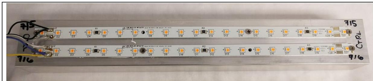
**Figure 2-5: Product NB-2 LED light engine consisting of two LED modules mounted on a common heat sink.**
