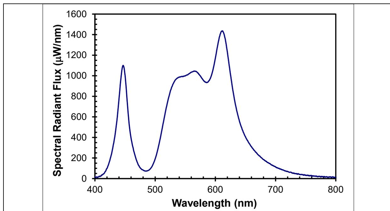
Figure 1-3: Emission spectrum of a photoluminescent nanofiber device containing a blue LED, a Ce:YAG phosphor, and red QDs [5]
