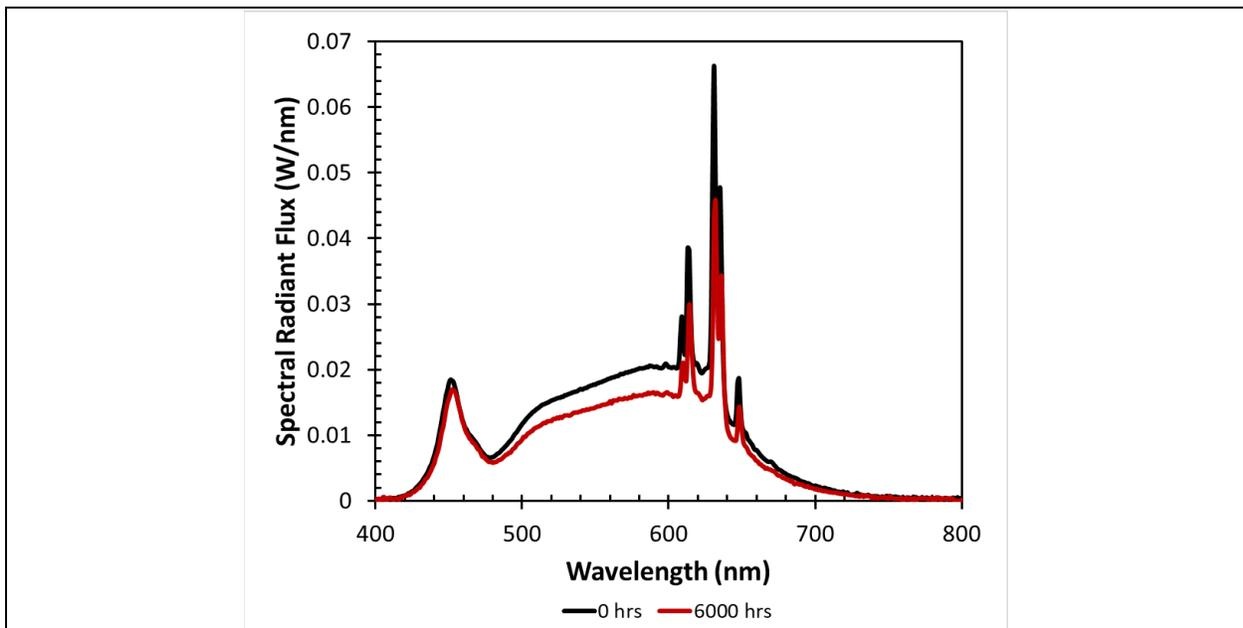
Figure 3-3: Spectral radiant flux for Product NB-1 at the beginning of testing and after 6,000 hrs of exposure during 7575.
