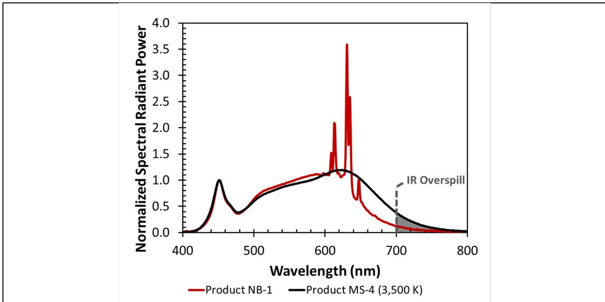
Figure 2-4: The SPD of Product NB-1 shows reduced IR emissions compared to Product MS-4. Emissions are normalized to the blue peak.
