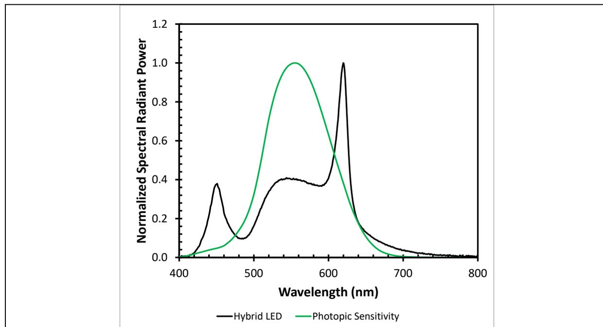
**Figure 1-2: Comparison of the wavelength dependence of a typical hybrid-LED device with the photopic sensitivity curve. The spectral power distribution (SPD) is normalized to a value of 1.0 for  $\lambda_{\max}$  [2].**
