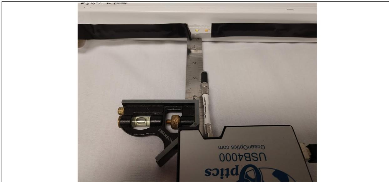
Figure 2-8: Absolute irradiance measurement setup for Product NB-1 pc-LEDs.
