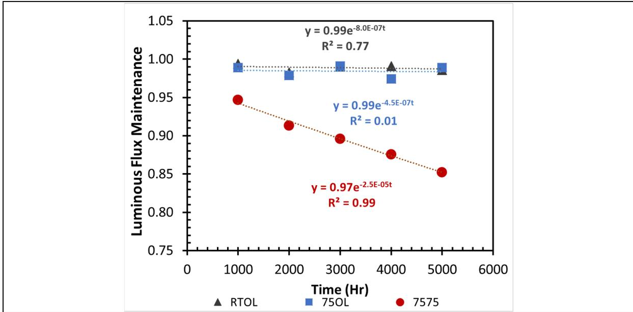
Figure 3-6: LFM of Product NB-2 during RTOL, 750L, and 7575 according to IES LM-84-14 and IES TM-28-14.
