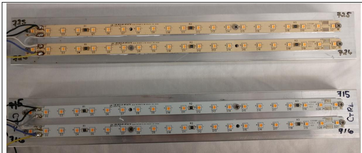
Figure 3-9: The control (bottom) and a tested LED module (top) after 5,000 hrs of exposure to the 7575 environment.
