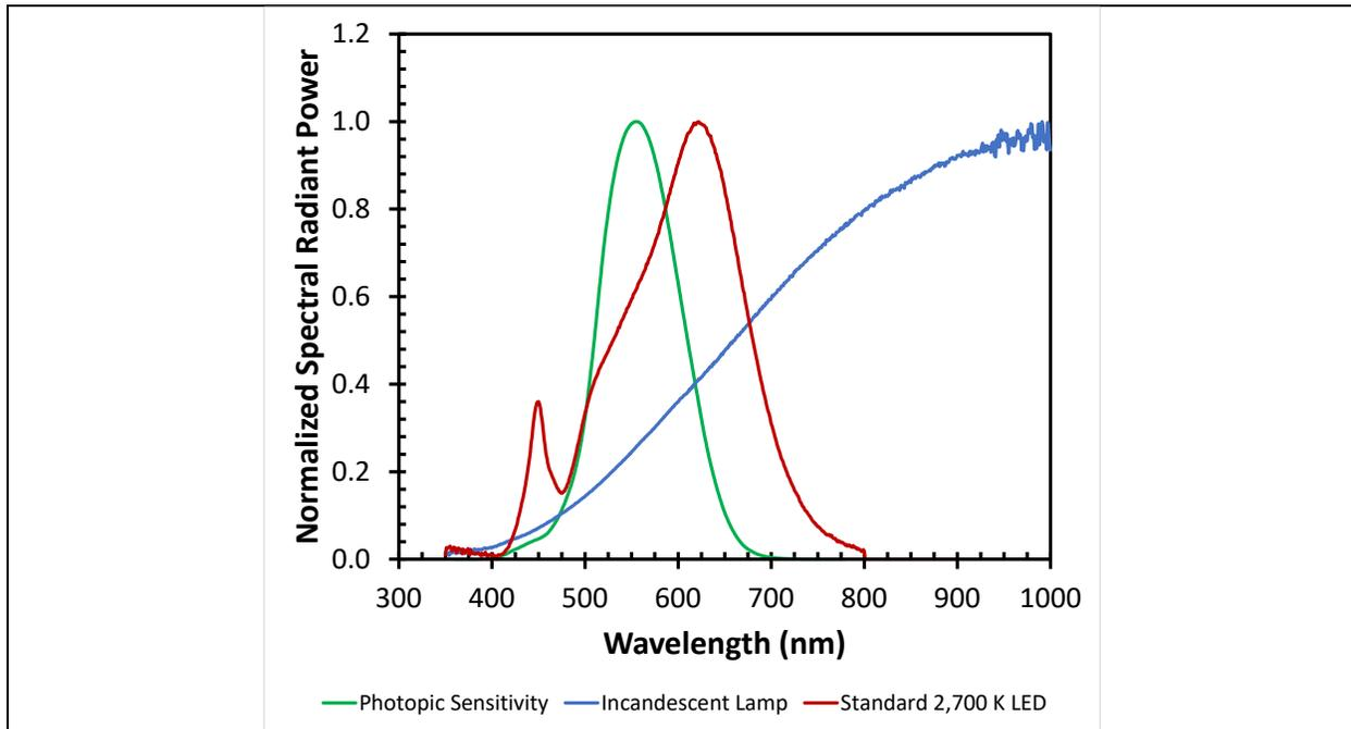
**Figure 1-1:** Comparison of the wavelength dependence of incandescent lamp emission, LED lamp emissions, and the photopic sensitivity curve. All spectra are normalized to a value of 1.0 for the maximum emission wavelength ( $\lambda_{max}$ )
