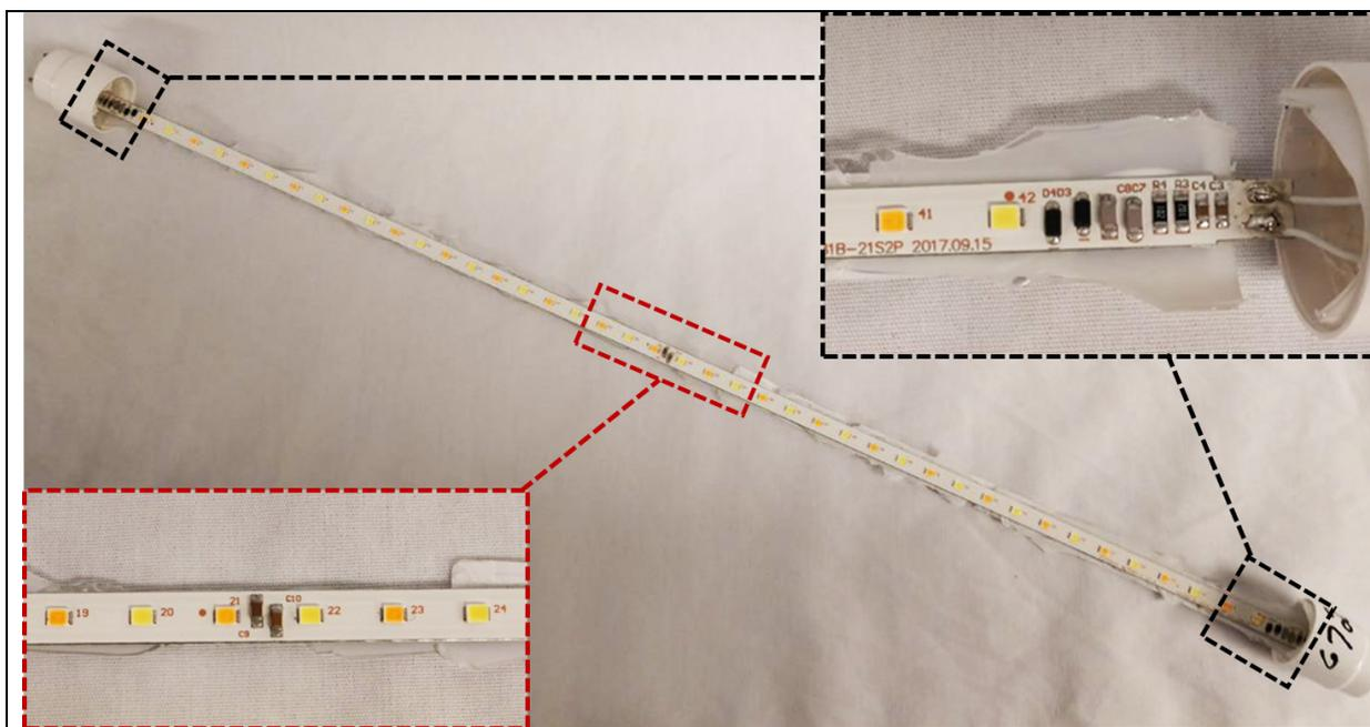
Figure 2-2: Product NB-1 with the glass globe removed. The black dotted inset shows the electronic circuitry on the PCB while the red dotted inset shows the arrangement of the LEDs and capacitors in the center of the LED module.
