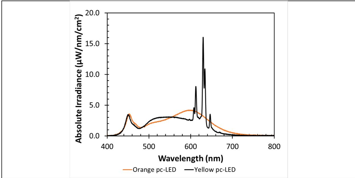
Figure 2-3: The absolute irradiance spectra of the pc-LEDs used in Product NB-1.
