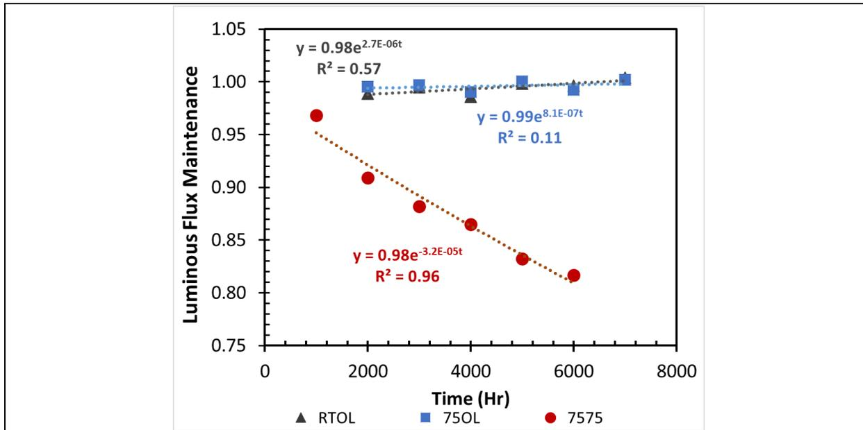
Figure 3-1: LFM of Product NB-1 during RTOL, 75OL, and 7575 according to IES LM-84-14 and IES TM-28-14.
