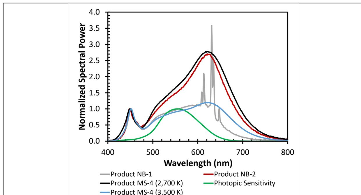
**Figure 4-1:** The normalized SPDs of the narrow-band red emitter products examined in this study compared to an all-phosphor product (MS-4) and the photopic sensitivity curve. The SPDs are normalized to the blue peak.
