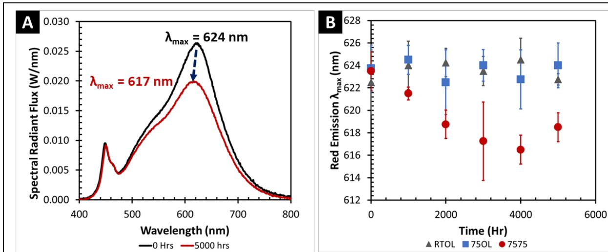
**Figure 3-8: Product NB-2 (A) SPD as initially measured and after 5,000 hrs of 7575 exposure and (B) average red emission peak maxima for the DUTs subjected to the different ASTs. The average red emission peak maxima in the 7575 conditions changed throughout testing while no noticeable change occurred in RTOL and 75OL environments, suggesting phosphor and QD oxidation and degradation was largest in the high humidity environment.**
