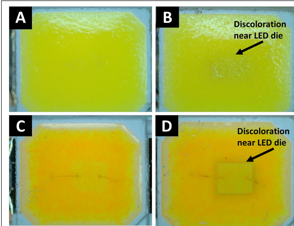
Figure 3-5: Selected LED primaries from the control (A and C) and an aged DUT operated in 7575 post-7,000 hrs (B and D) for Product NB-1. The aged DUT shows discoloration near the LED die (B and D).
