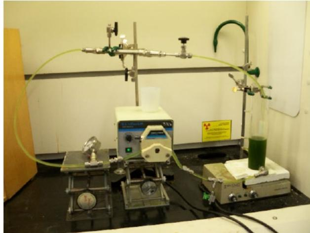
Recirculating Membrane Test System
