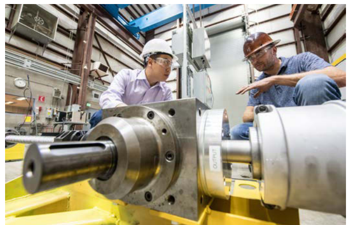
NREL researchers test the power take-off system on a dynamometer designed for wave energy conversion at NREL's Flatirons Campus.
