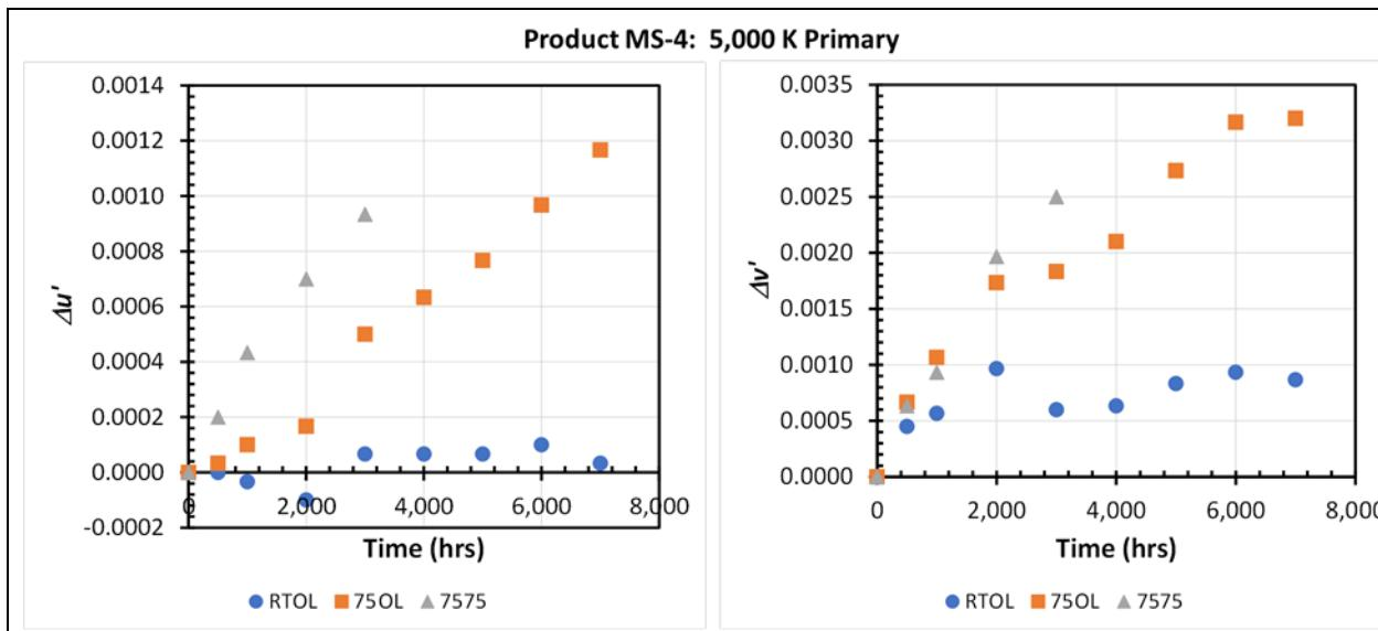
Figure A-10: Temporal change in  $\Delta u'$  and  $\Delta v'$  from the 5,000 K primary of Product MS-4 in different AST environments.
