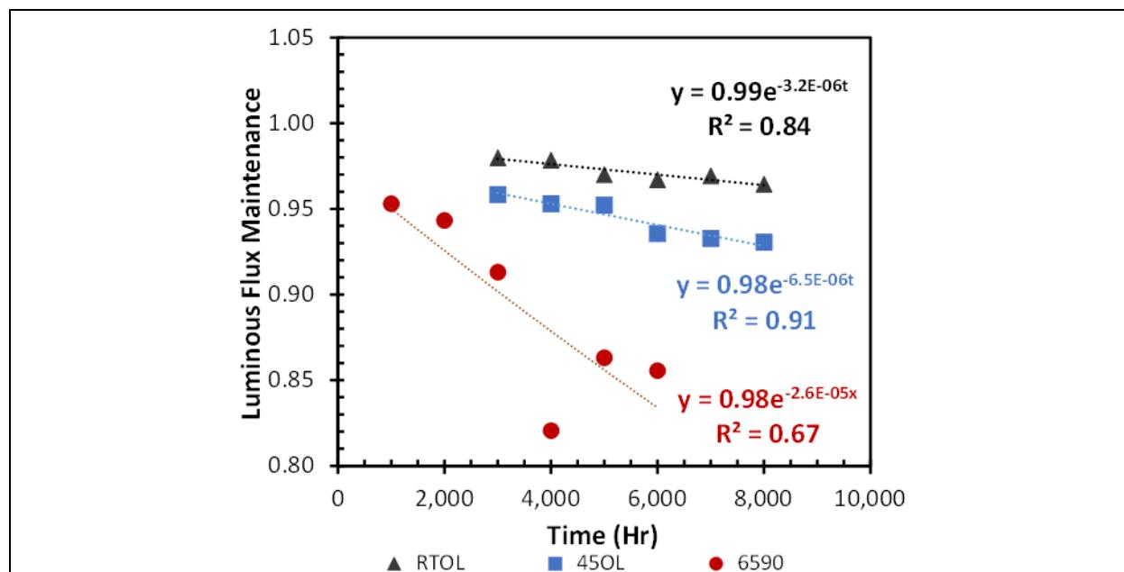
Figure 3-1: LFM of Product MS-1 during RTOL, 45OL, and 6590 according to IES LM-84-14 and IES TM-28-14.
