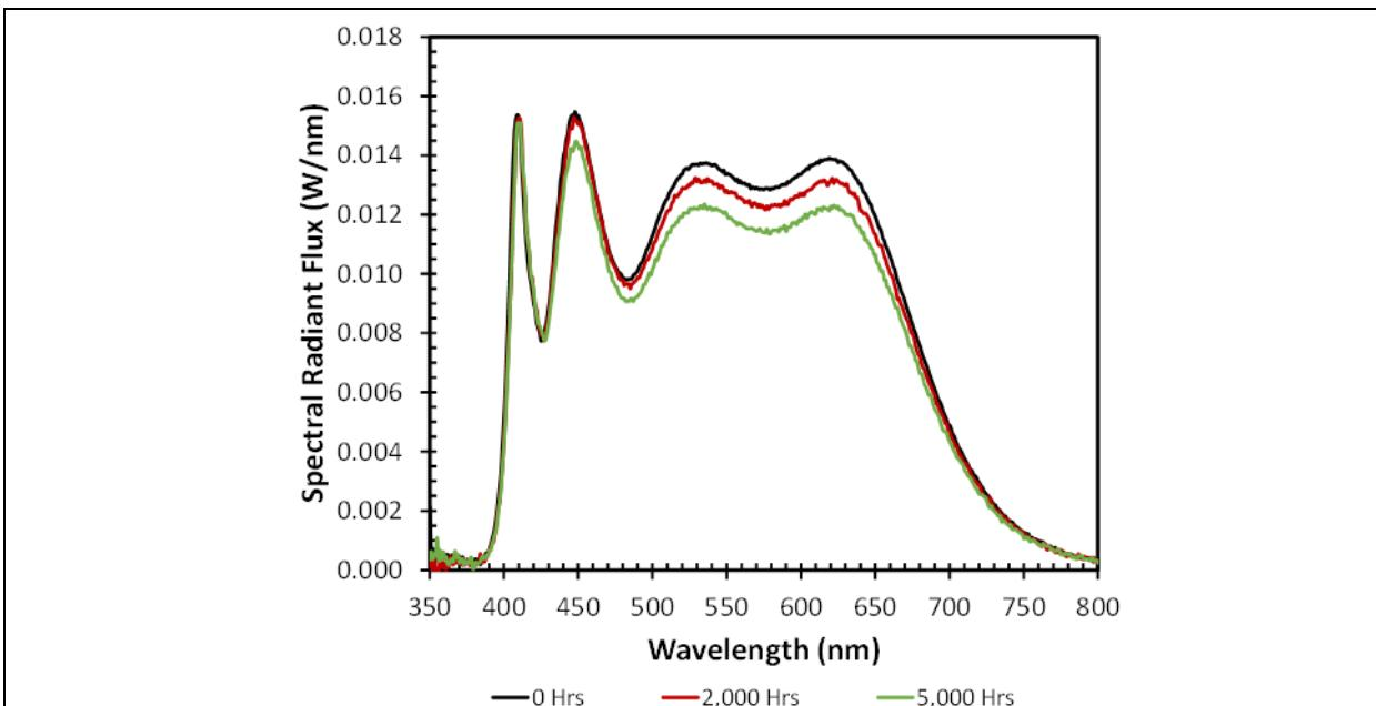
Figure 3-16: SPDs for Product MS-3 operated during 750L for various times.
