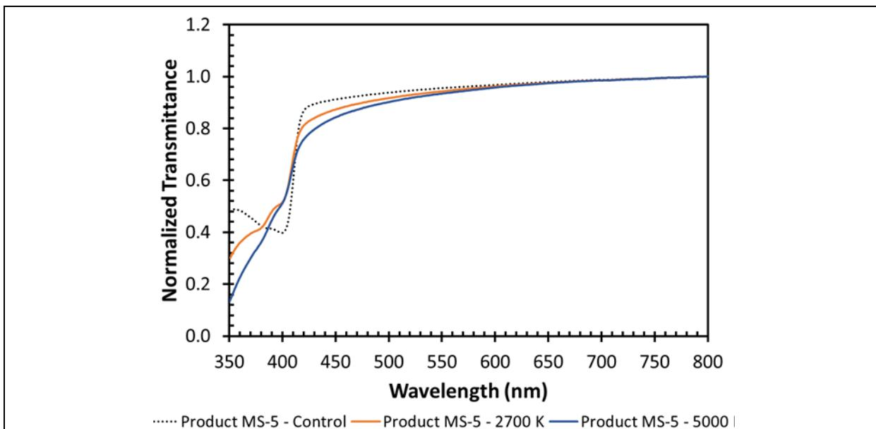
Figure 3-31: Transmittance data (normalized at 800 nm) for Product MS-5 lenses show less transmittance at high energy wavelengths after AST.
