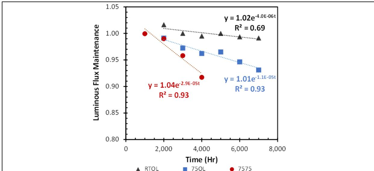
Figure 3-21: LFM of the Product MS-4 test populations operated with the 5,000 K primary. Testing was performed in RTOL, 75OL, and 7575.
