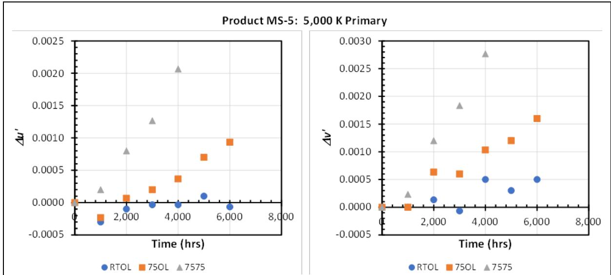
Figure A-12: Temporal change in  $\Delta u'$  and  $\Delta v'$  from the 5,000 K primary of Product MS-5 in different AST environments.
