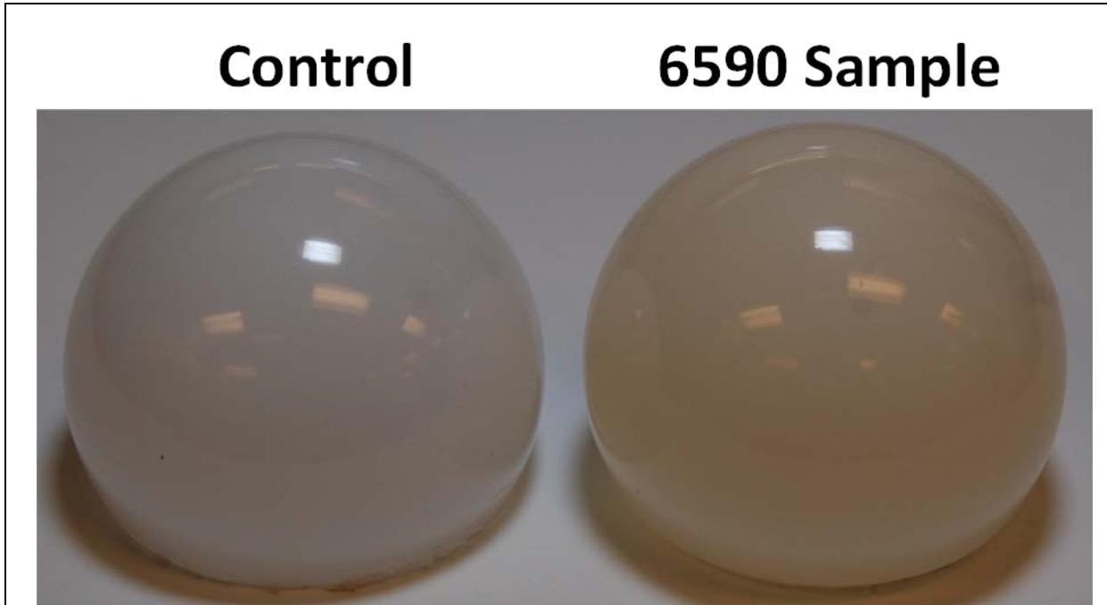
Figure 3-12: Product MS-2 after 6,000 hrs of 6590 testing compared with a control sample.
