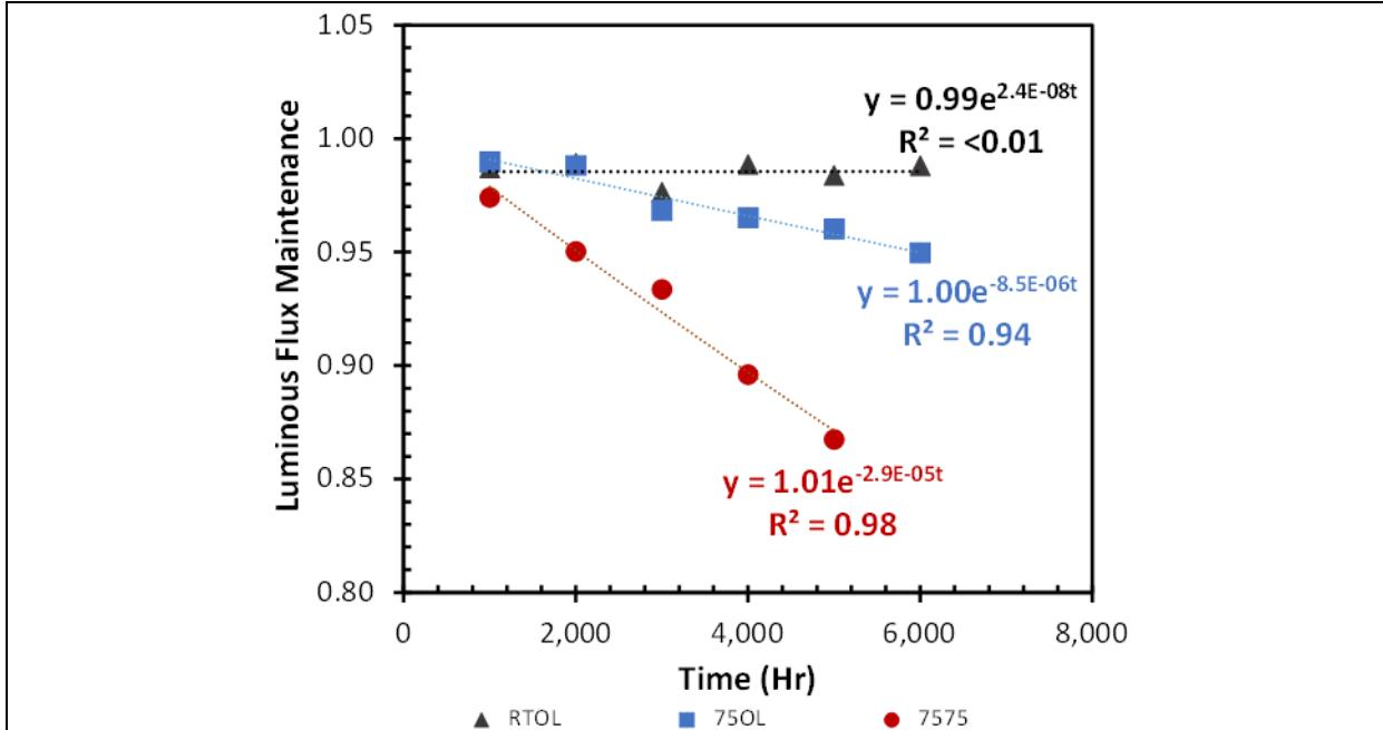
Figure 3-26: LFM of the 2,700 K primary for Product MS-5 in different AST protocols.
