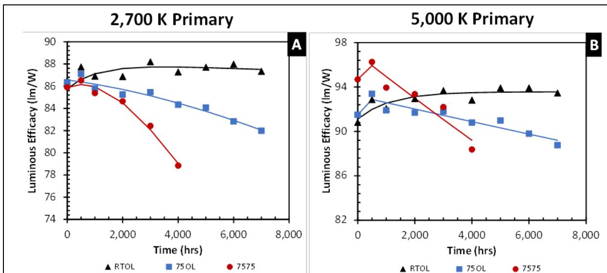
Figure 3-22: Temporal change in luminous efficacy for Product MS-4: (A) for the 2,700 K primary and (B) for the 5,000 primary.
