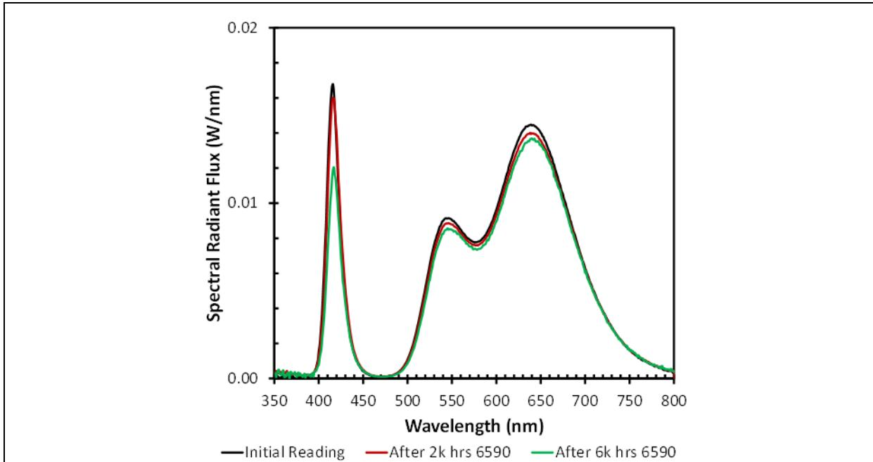
**Figure 3-9:** SPD of Product MS-2 as initially measured, after 2,000 hrs of 6590 exposure, and after 6,000 hrs of 6590 exposure.
