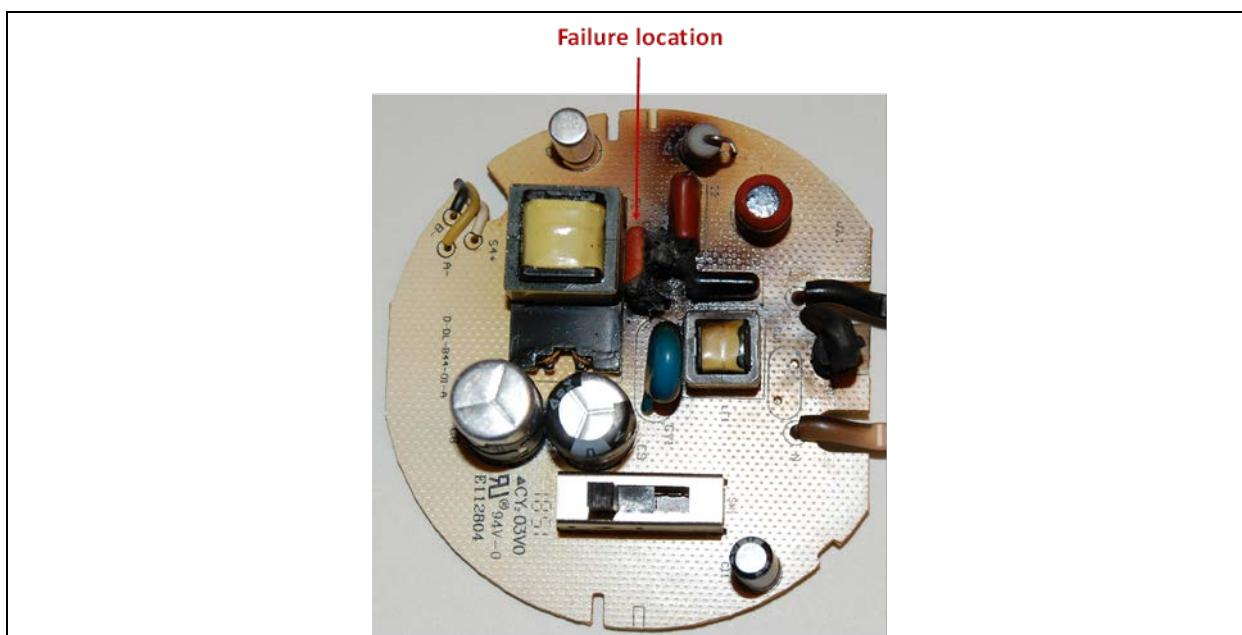
Figure 3-24: Failed driver from Product MS-4 after 5,000 hrs of 7575.
