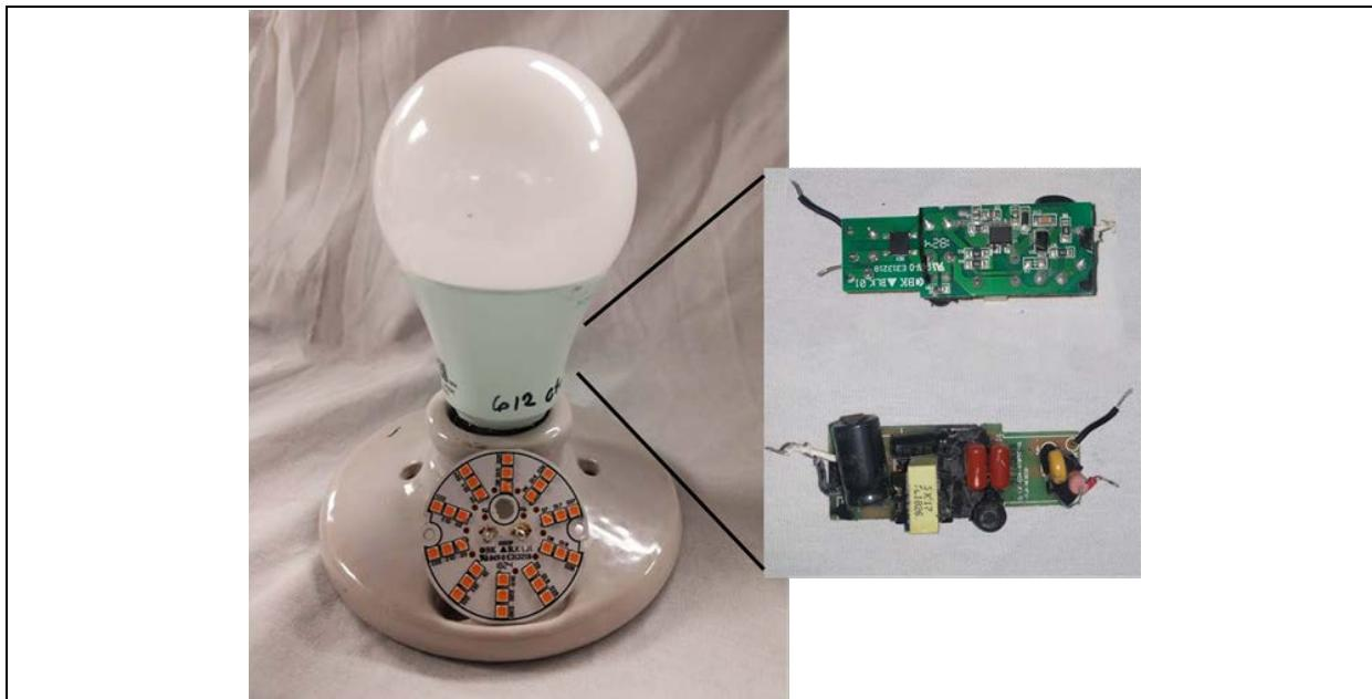
Figure 2-4: (On left) Product MS-2 with the globe, but in an unenergized state, along with the LED module.
