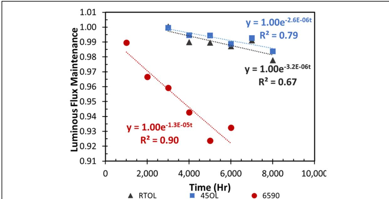
Figure 3-6: LFM of Product MS-2 during RTOL, 450L, and 6590 according to IES LM-84-14 and IES TM-28-14.
