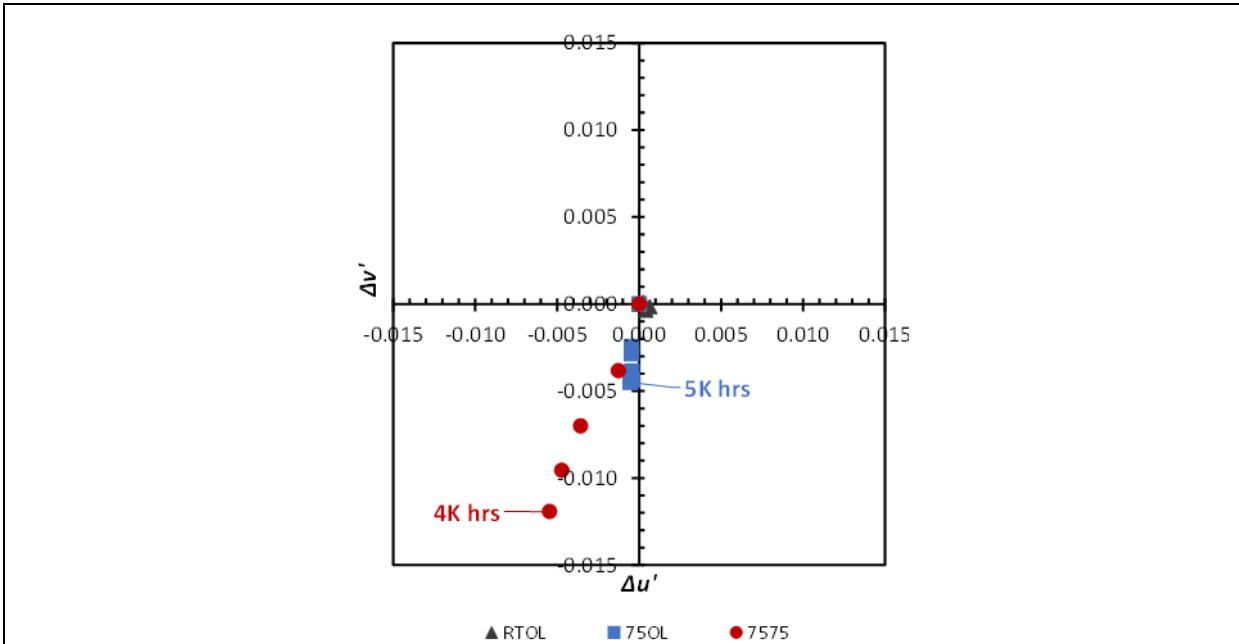
Figure 3-15: Chromaticity shift diagram for Product MS-3 in RTOL, 750L, and 7575.
