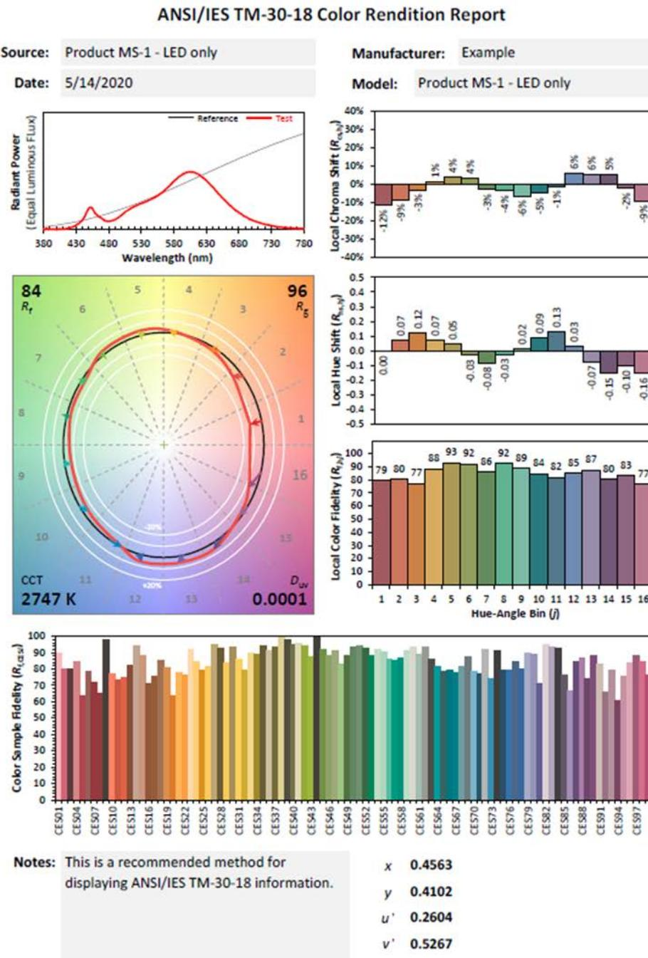
Figure A-2: ANSI/IES TM-30-18 analysis for LEDs from Product MS-1 without the glass globe.
