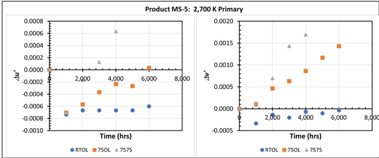
Figure A-11: Temporal change in  $\Delta u'$  and  $\Delta v'$  from the 2,700 K primary of Product MS-5 in different AST environments.
