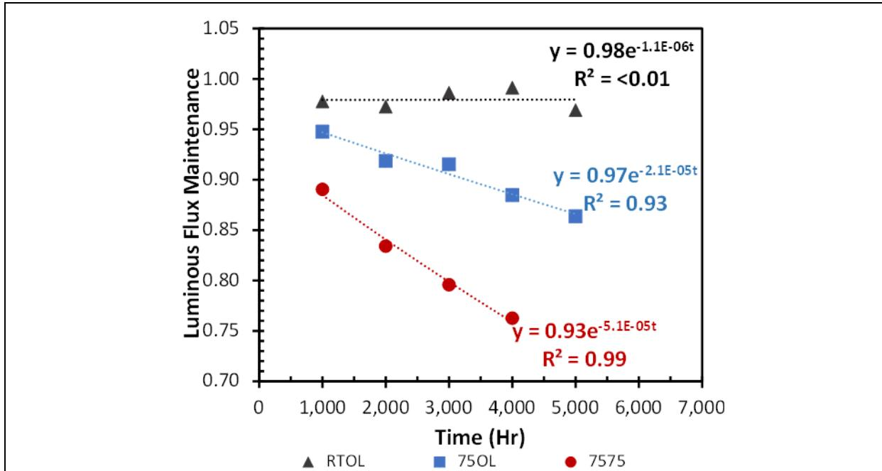
Figure 3-13: LFM for Product MS-3 during RTOL, 750L, and 7575 according to IES LM-84-14 and IES TM-28-14.
