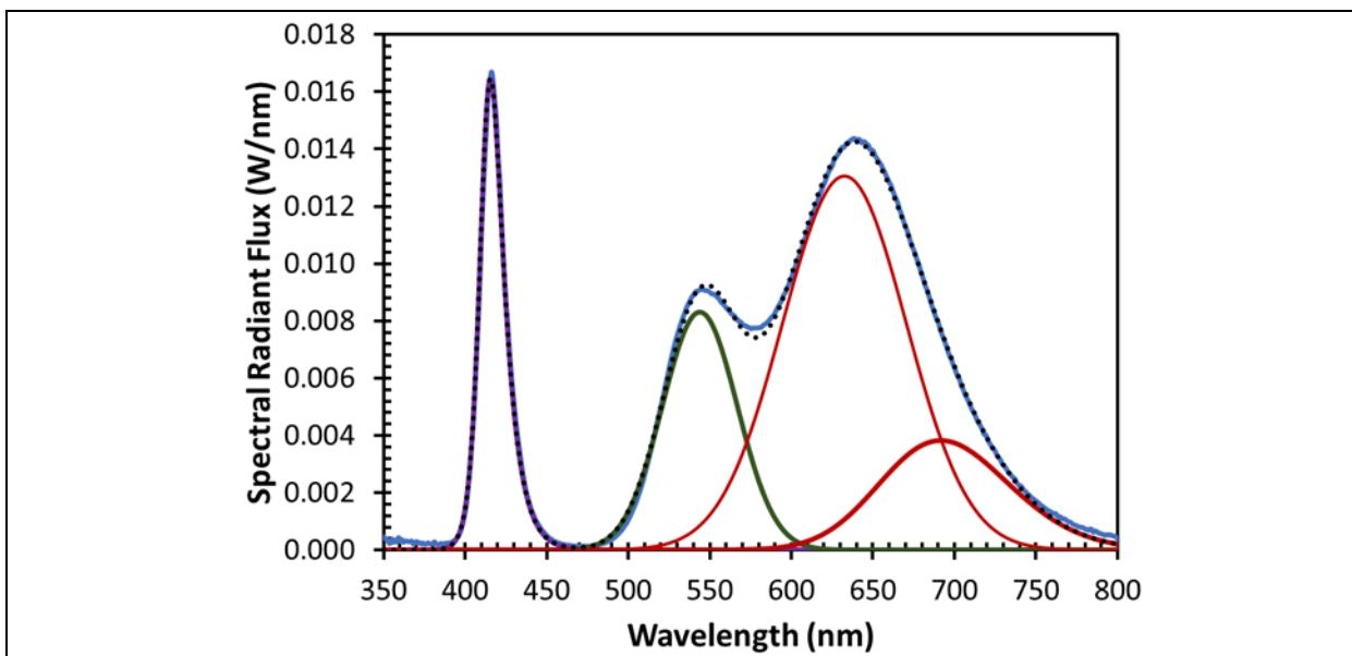
**Figure 3-10:** Spectral deconvolution of the initial emissions from Product MS-3.
