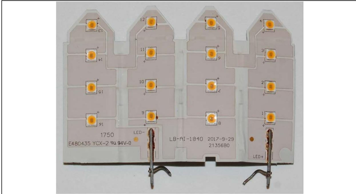
Figure 3-5: LED module from Product MS-1 after 7,000 hrs of 6590.
