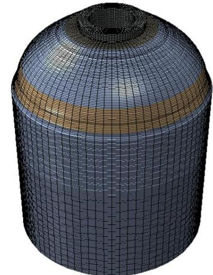
A 3D model for a H<sub>2</sub> cryo-compressed pressure vessel
