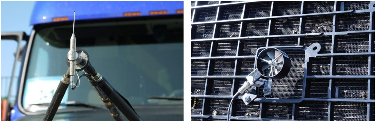
**Figure 3-6. Supplemental airflow instrumentation from truck platooning experiments: (left) Cobra probe mounted 1 meter ahead of vehicle and 2 meters off the ground, (right) air velocity transmitter mounted flush to center of grill.**
