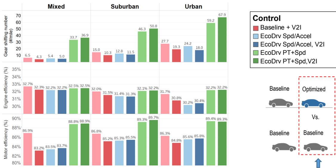
Figure 3-95. Various component operation metrics for the HEV in a lead position (current technology).
