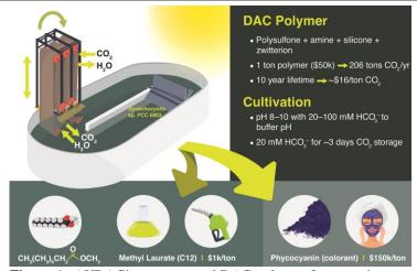
**Figure A**. AUDACity uses a novel DAC-polymer for capturing CO<sub>2</sub> from air and directly delivering to a culture of photosynthetic microbes at scale for producing sustainable fuels and valuable products, such as methyl laurate and phycocyanin.
