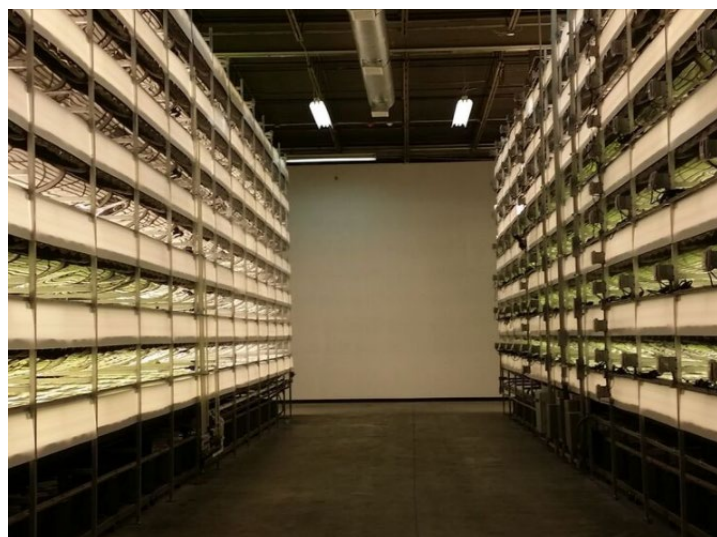
Figure 2-3 A Vertical Farm Growth Configuration; AeroFarms in Newark, NJ. Vertical stacking the grow areas of leafy greens and herbs enable the total grow area of a facility to be increased in the same building footprint. [6]
