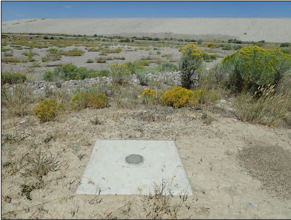
PL-7. Quality Control Monument and Ancillary Cell with Disposal Cell South Side Slope in Background
