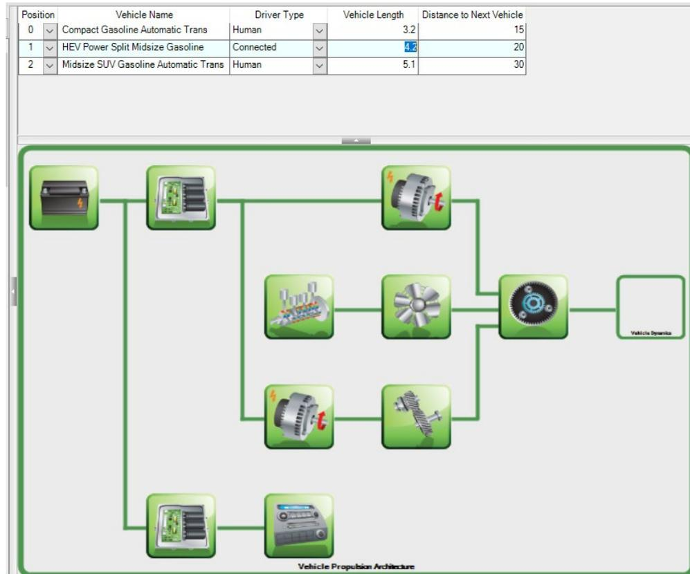
Figure I.6.2.5 RoadRunner user interface based on AMBER framework
