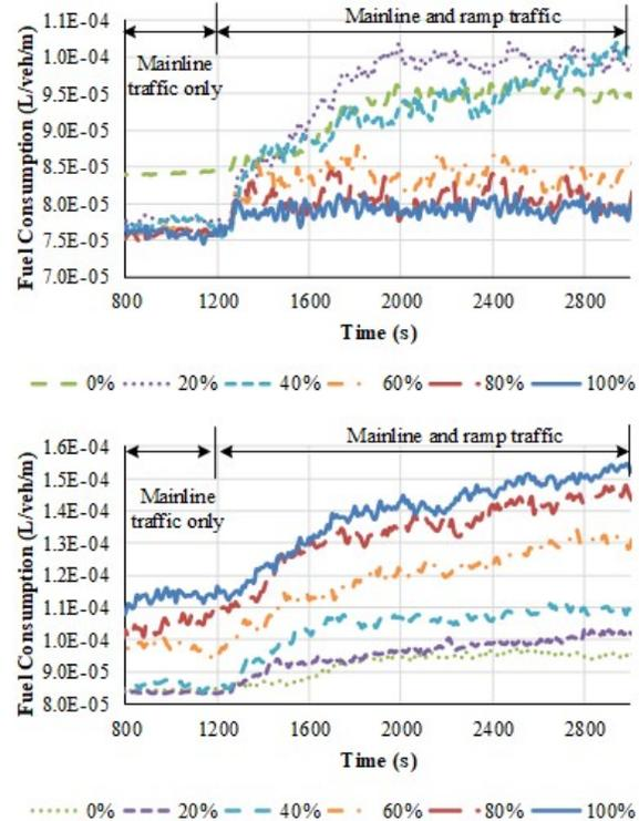
Figure 2 Time Series of Fuel Consumption Impacts of ACC and CACC Vehicles (Upper graph is for CACC cases, Lower graph is for ACC Cases)
