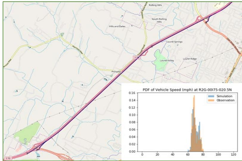
Figure I.2.4.3. Corridor modeled in VISSIM and histogram of observed vs simulated vehicle speeds in the 20.5 N mile marker
