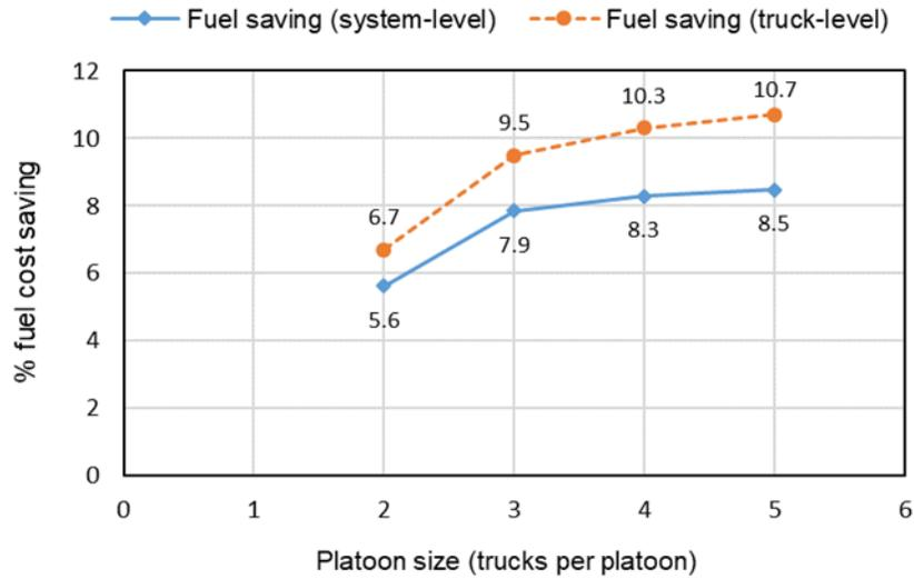
Figure I.4.1.6 Impact of platoon size on fuel cost savings
