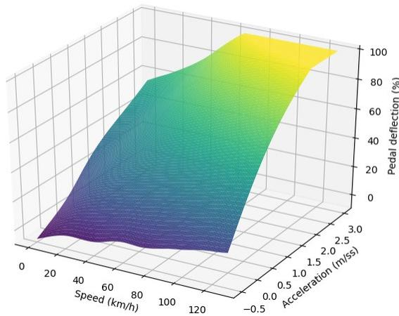
Figure I.2.7.4 Accelerator pedal map for 2017 Toyota Prius Prime
