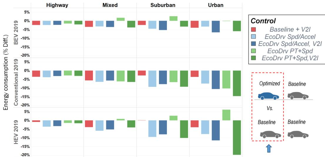
Figure I.2.3.7 Energy consumption of following vehicle (control versus baseline) with current technology and various powertrains
