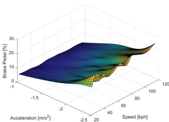
Figure I.2.7.12 Brake pedal map for 2014 Honda Accord
