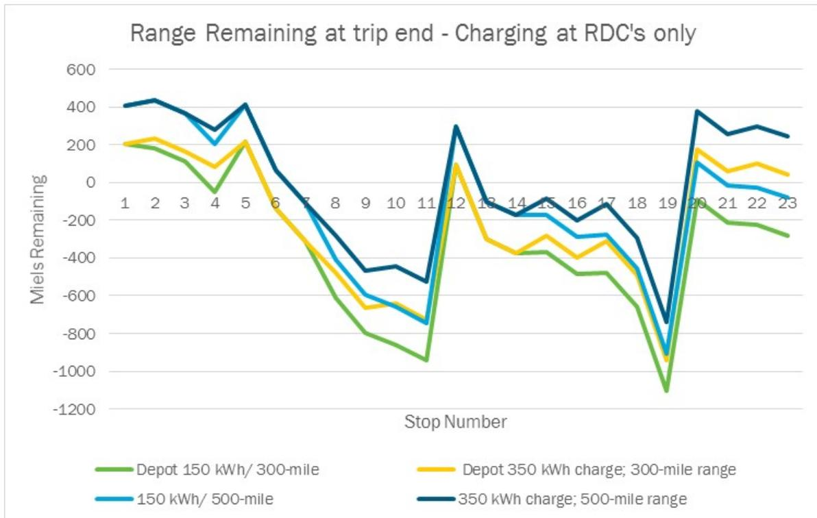
Figure I.1.4.6 Range remaining at each stop for depot only charging
