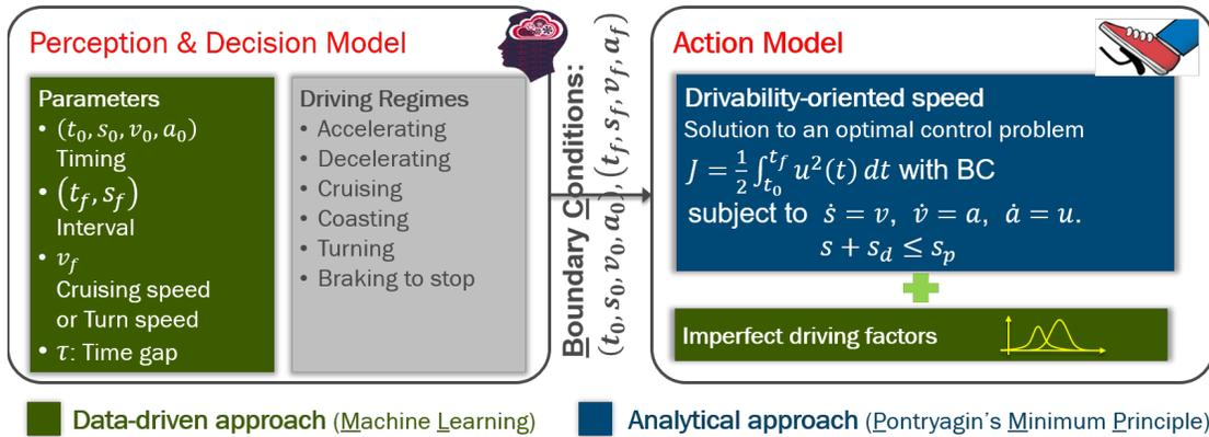
Figure I.2.3.2 Schematic diagram of the human driver model: P&D model [left] and action model [right]
