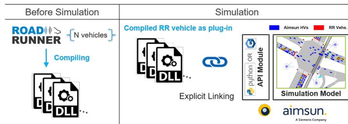
Figure I.6.3.4 Structure using Aimsun microSDK to link RoadRunner to Aimsun
