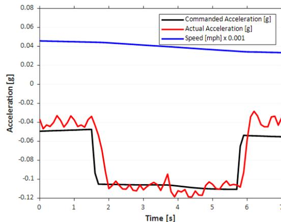
Figure I.2.7.13 Brake system response to brake pedal override on 2014 Honda Accord
