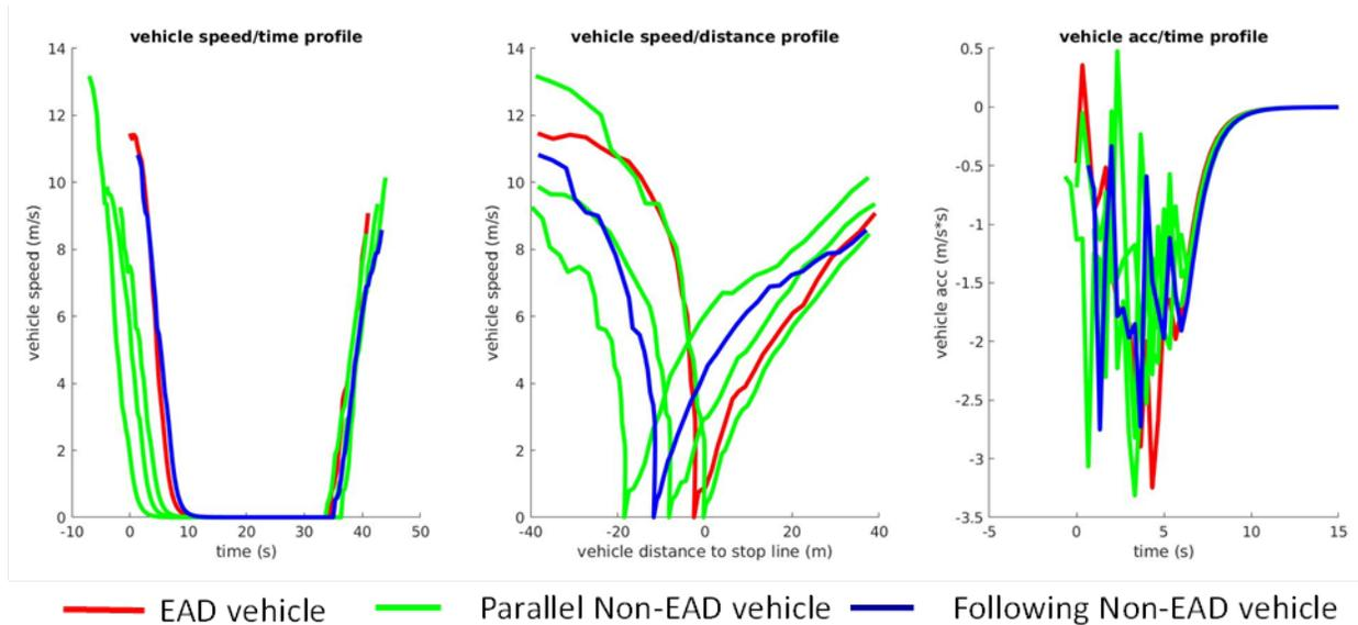
Figure I.2.8.8 EAD Case IV: EAD trailed behind from no-EAD vehicles travel in the adjacent lane
