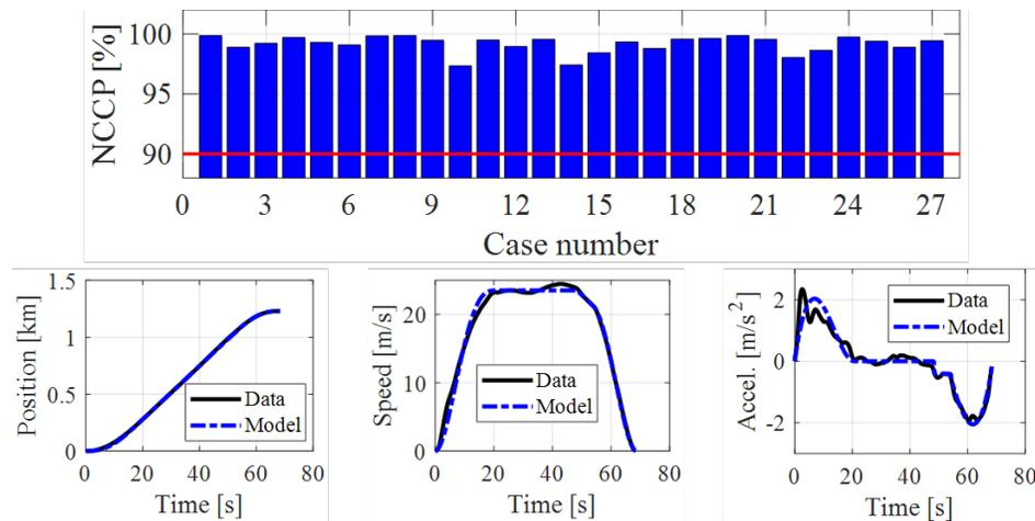
Figure I.2.3.3 Normalized cross correlation power (NCCP) between experimental and simulation data for 27 segments [top] and for one sample [bottom].
