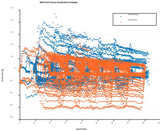
Figure I.2.7.6 ACC override acceleration envelope for 2013 Ford Taurus
