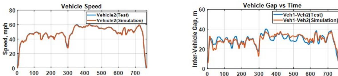
Figure I.2.3.1 Comparison of the adaptive cruise control model in RoadRunner with test data
