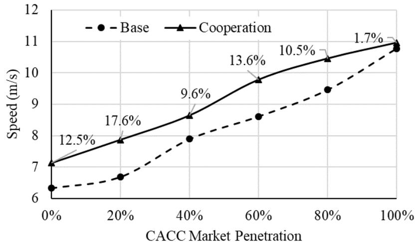
Figure I.2.1.8 Average vehicle speed under various CACC market penetrations
