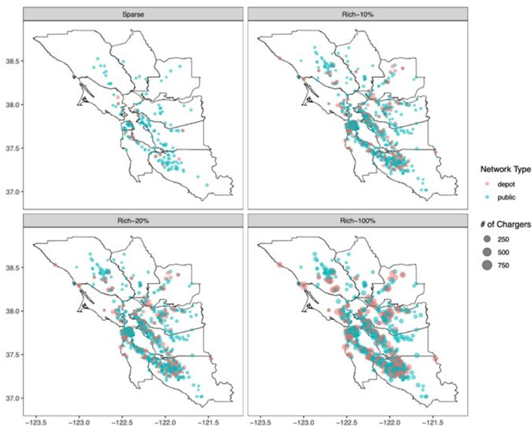
Figure I.1.2.7 Spatial distribution of chargers in San Francisco Bay Area by network type. “Depot” chargers are exclusively available to fully automated, driverless ride-hailing vehicles while “public” chargers are shared between ride-hailing and personal-use EV drivers.
