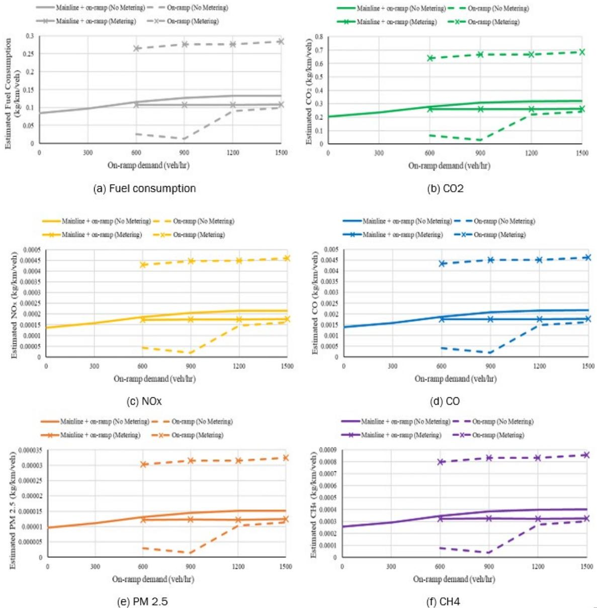
Figure I.2.1.10 Emission and fuel consumption estimates at varying levels of on-ramp demand
