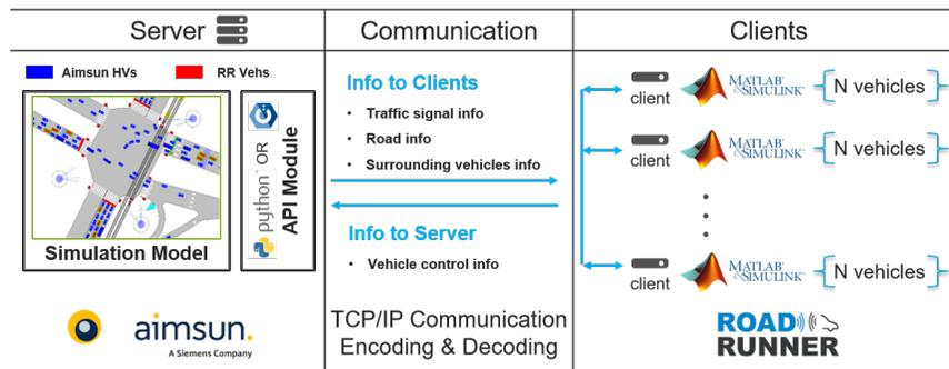
Figure I.6.3.3 Structure using Aimsun microAPI to link RoadRunner to Aimsun
