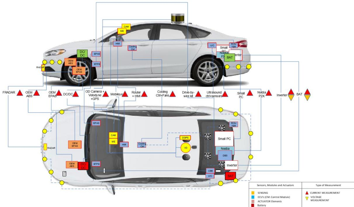
Figure I.2.9.2 Ford Fusion HEV (FEV AV Demonstrator) Instrumentation Overview
