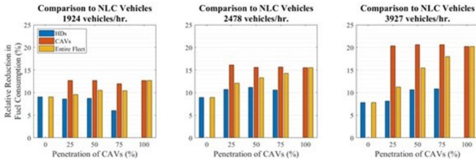
Figure 9 Percent Reduction in Fuel Consumption by Flow Rate and Penetration
