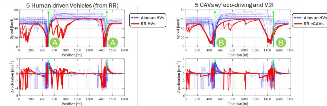
Figure I.6.3.7 Speed and acceleration trajectory of five RoadRunner vehicles [solid red lines], which are either human-driven vehicles [left] or eco-driving CAVs [right], and default Aimsun human-driven vehicles [dotted blue lines]
