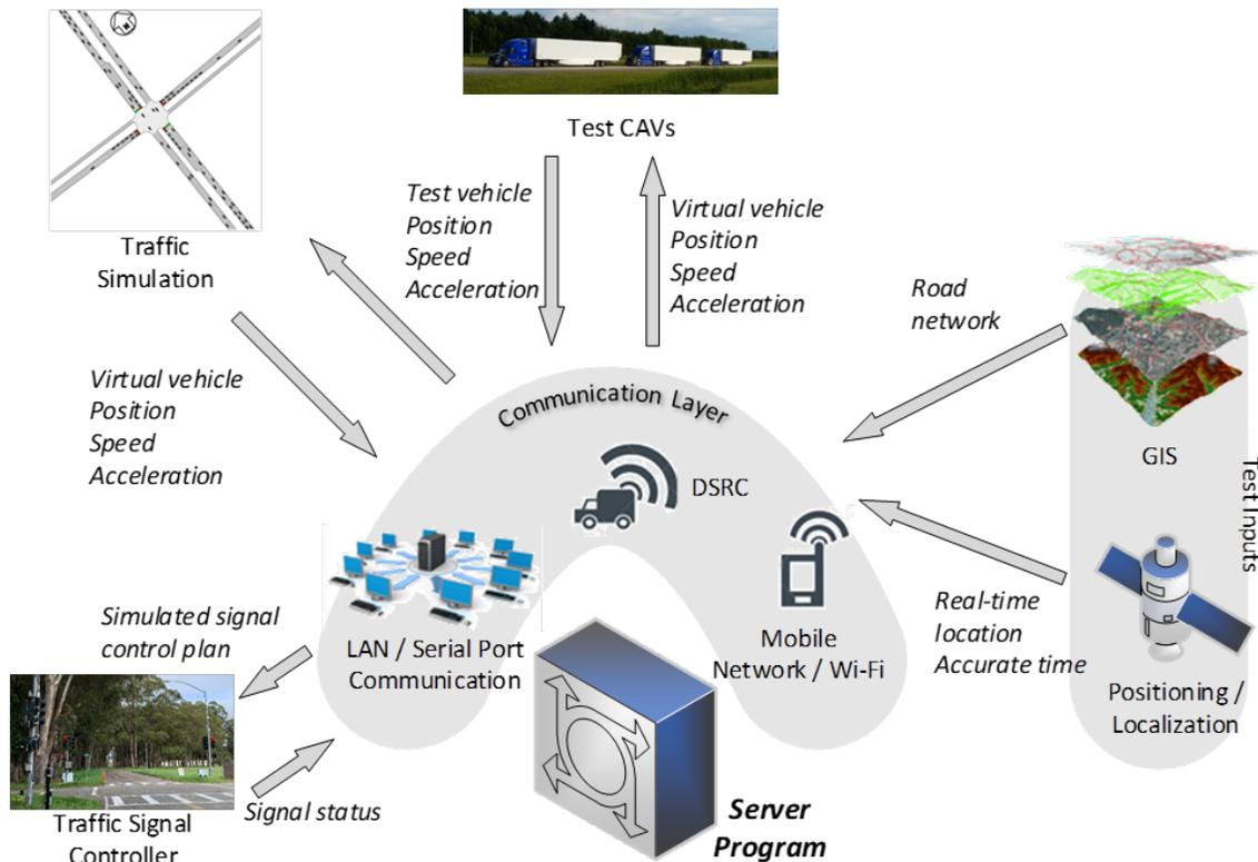
Figure I.2.6.1 Components and Data Flow of the Presented HIL Testbed
