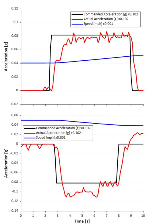
Figure I.2.7.7 Powertrain response to ACC acceleration override for 2013 Ford Taurus
