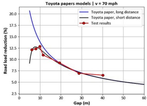
Figure 11 Road-Load Data from Second Vehicle in Two-Vehicle Platoon
