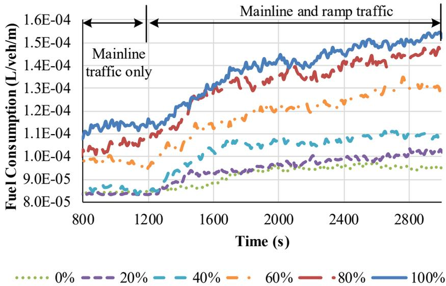
Figure I.2.1.4 Time series of fuel consumption rate under various CACC and ACC market
