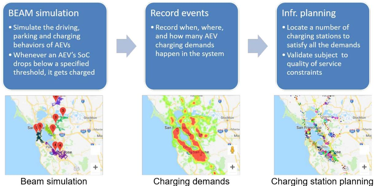
Figure I.1.2.2 FCSPlan and BEAM integration
