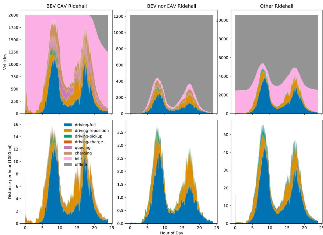
Figure I.1.2.12 Distribution of the ride-hailing fleet into operating states over the 24-hour simulation period for scenario with 100 mile range EVs and Rich, 50kW charging infrastructure. Horizontal panels separate vehicle types and vertical panels separate time spent by each vehicle (top) and distance traveled by all vehicles (bottom).
