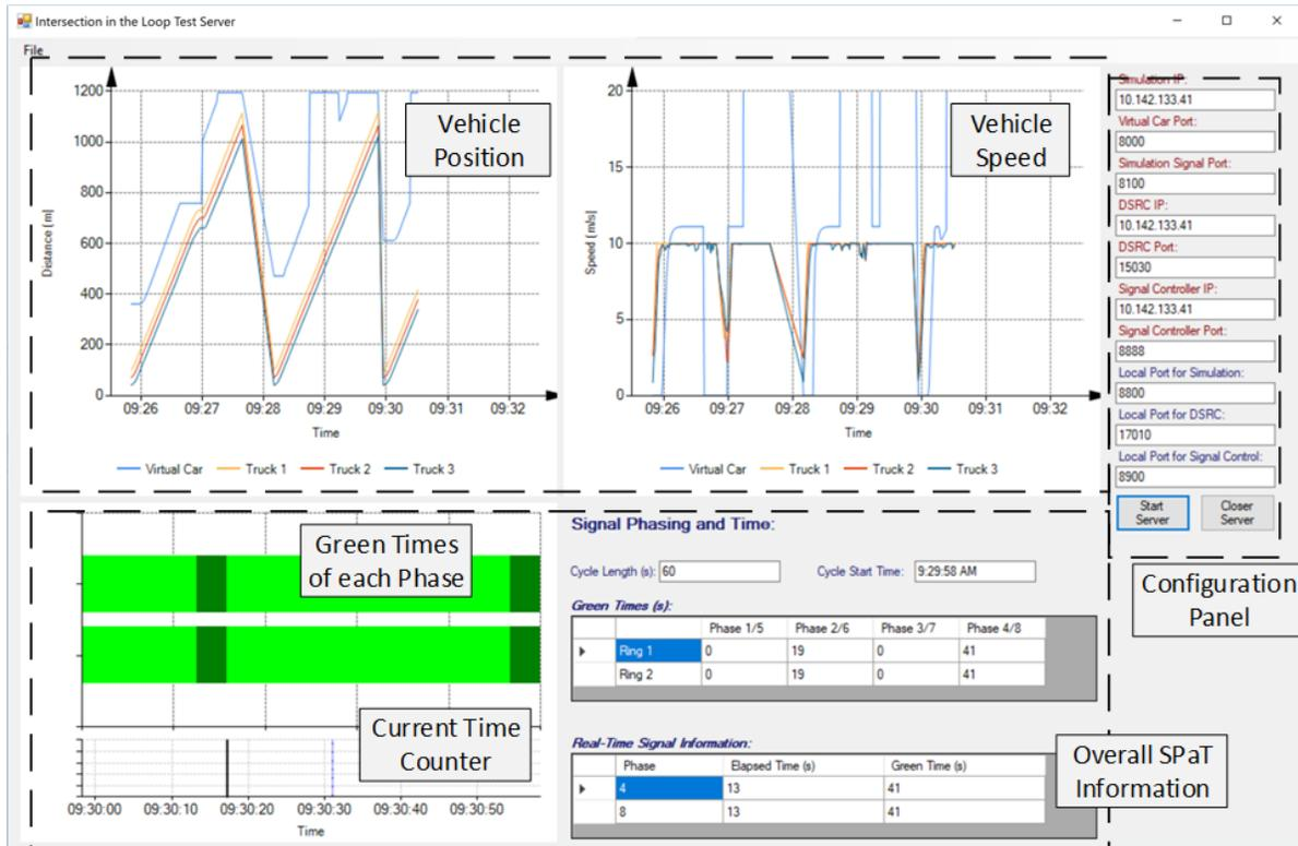
Figure I.2.6.4 Snapshot of the Server Program
