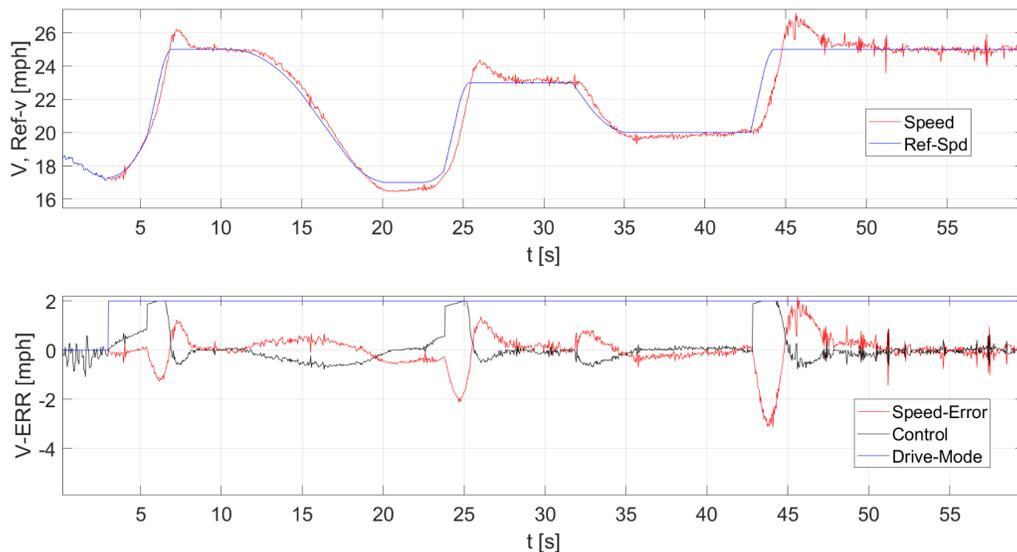
Figure I.2.7.17 Speed tracking directly using the ACC command from the upper level control: upper – reference speed (blue) and measured speed (red); lower: speed tracking error, acceleration control command, and drive mode (0-manual; 2-automatic control)
