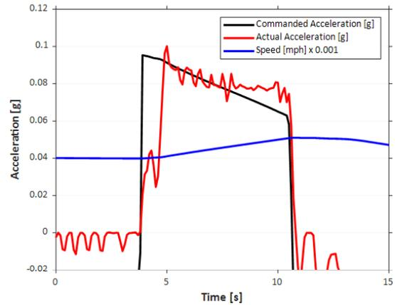
Figure I.2.7.9 Powertrain response to accelerator pedal override on 2013 Ford Taurus
