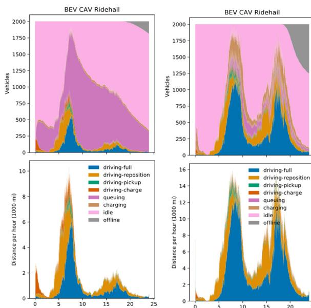
Figure 1 Operation State of Automated Ride-Hail BEVs with Sparse (left) and Rich (right) Charging Infrastructure
