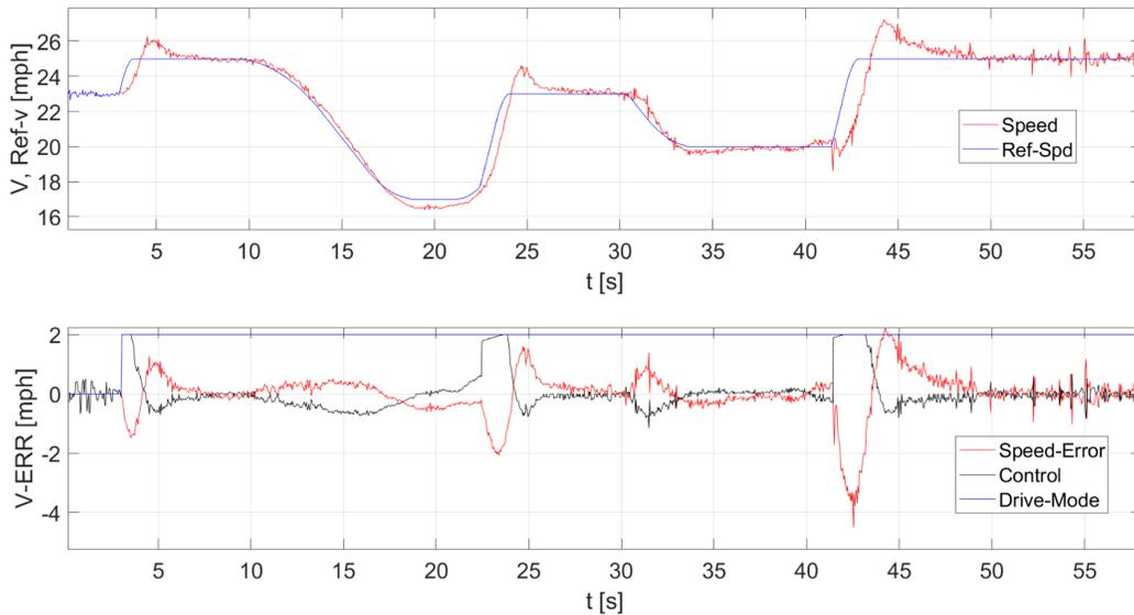
Figure I.2.7.16 Speed tracking using the torque mapping developed from the dynamometer test: upper – reference speed (blue) and measured speed (red); lower: speed tracking error, acceleration control command, and drive mode (0-manual; 2-automatic control)
