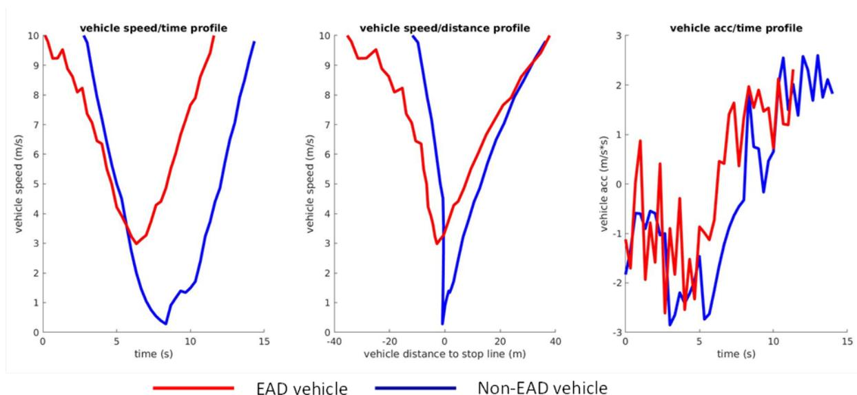
Figure I.2.8.4 Case of scenario 1: EAD Case I: EAD vehicle slows down but does not make full stop. Non-EAD vehicle nearby makes nearly a full stop (from left to right speed, speed vs distance to intersection, deceleration)
