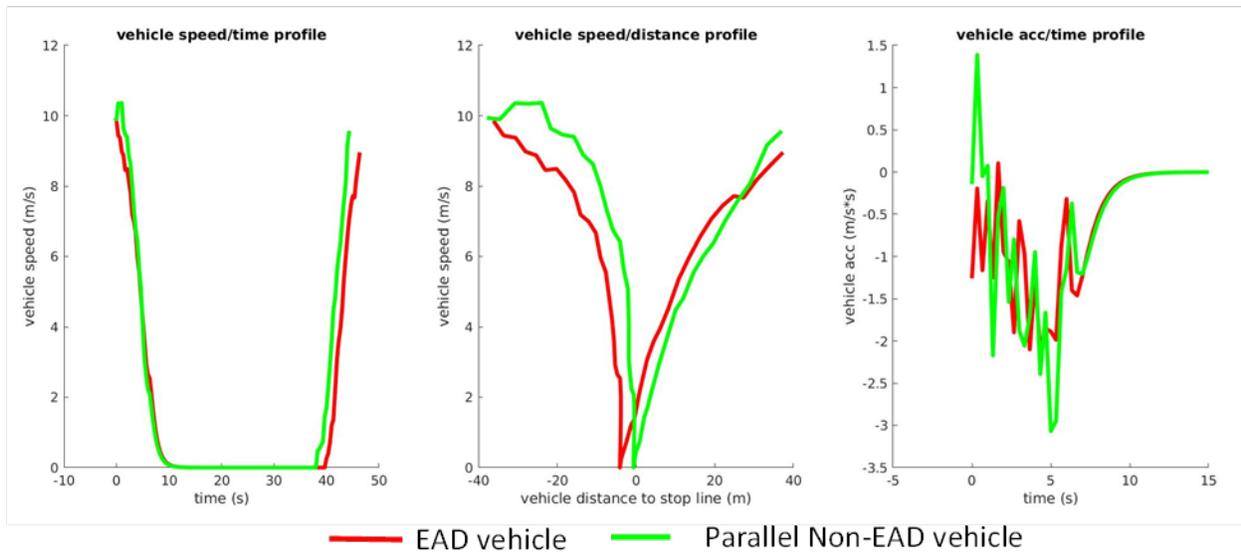
Figure I.2.8.7 EAD Case III: EAD and no-EAD vehicles travel in adjacent lanes and arrives at intersection as similar time
