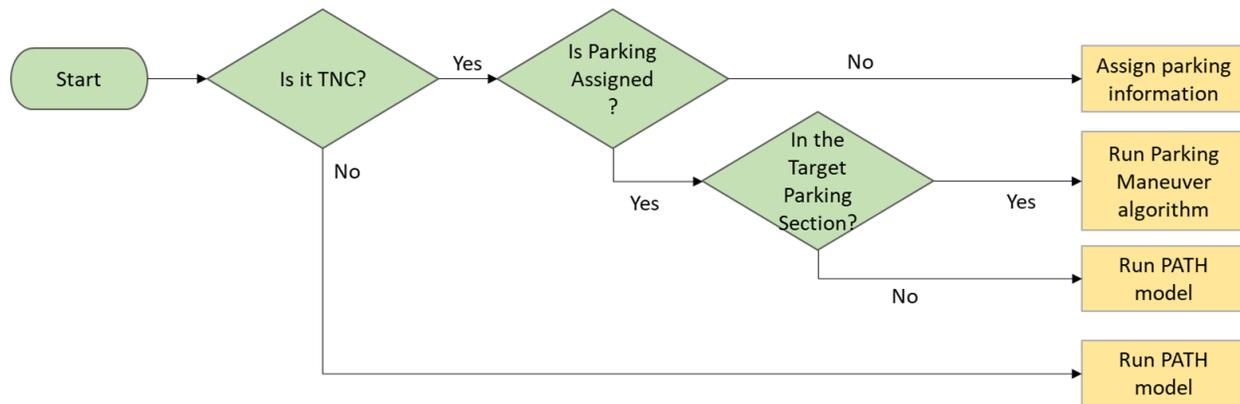
Figure I.6.1.1 The Framework for the Model of TNC Parking Maneuver with PATH Model
