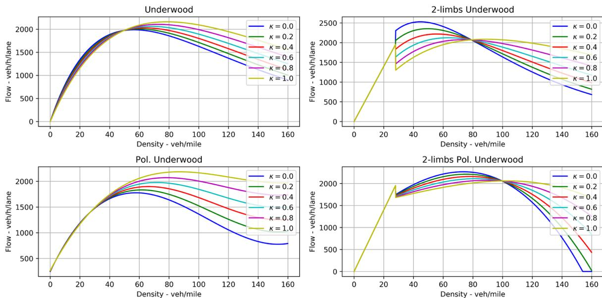
Figure I.2.2.3 Calibrated fundamental diagrams for the four models with varying penetration rates
