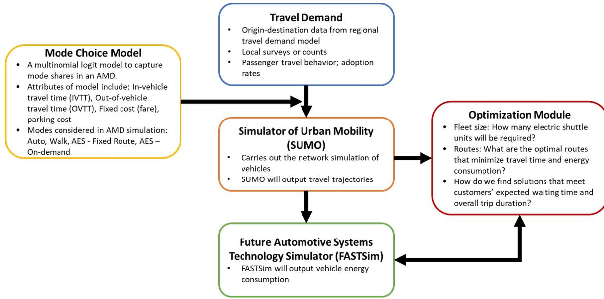
Figure I.5.6.1 Workflow of the AMD Modeling and Simulation Toolkit
