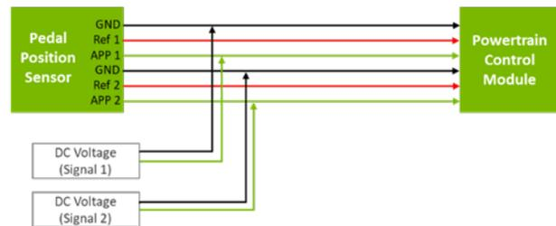
Figure I.2.7.15 Pedal override DC voltage injection diagram
