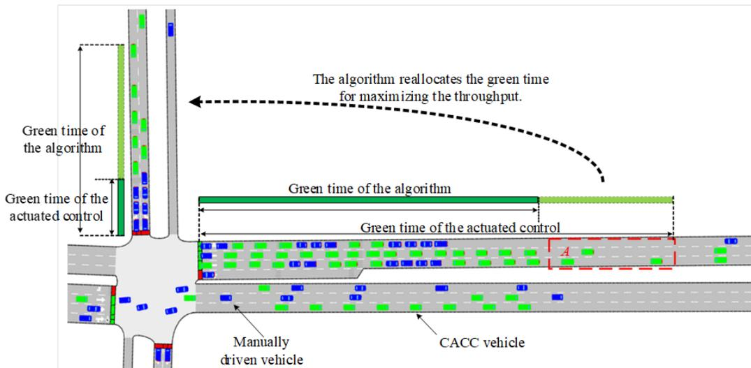
Figure I.2.1.1 Comparison of the proposed algorithm and actuated control
