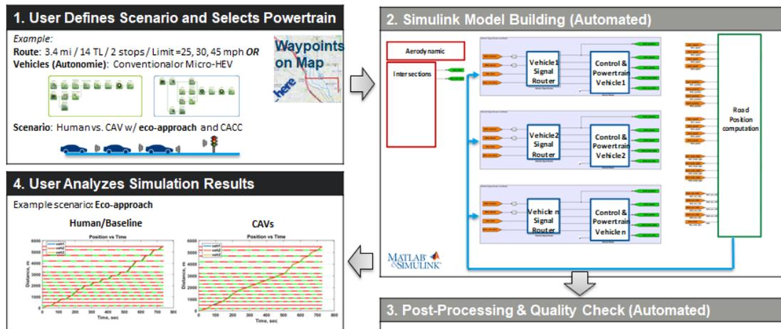
Figure I.6.2.2 RoadRunner workflow to simulate a CAV scenario
