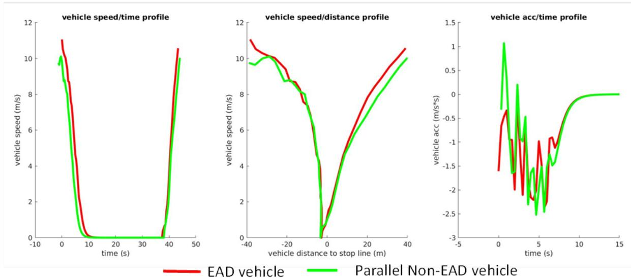
Figure I.2.8.6 EAD Case II: EAD and no-EAD vehicles travel in adjacent lanes and arrives at intersection as similar time
