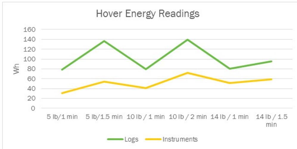
Figure I.4.2.2 Energy estimates from internal logs versus external instruments (INL)
