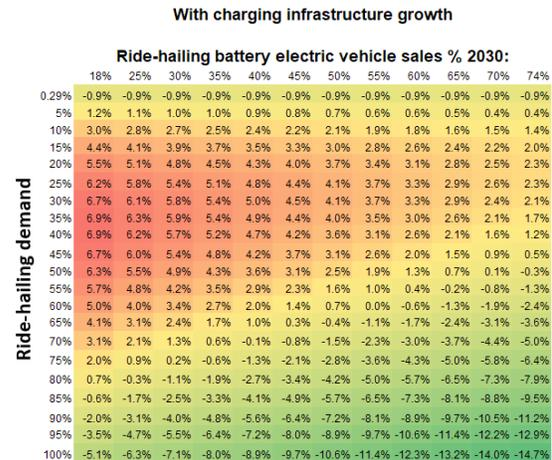
Figure I.1.1.4 National carbon emission reduction (shown as percentages, original unit is Million Metric Tons of Carbon Equivalent or MMTc) as a function of ride-hailing demand, BEV market penetration, and charging infrastructure. Green means a reduction, yellow means relatively no change, and red means an increase. (Carbon emissions include emissions from upstream and vehicle use)
