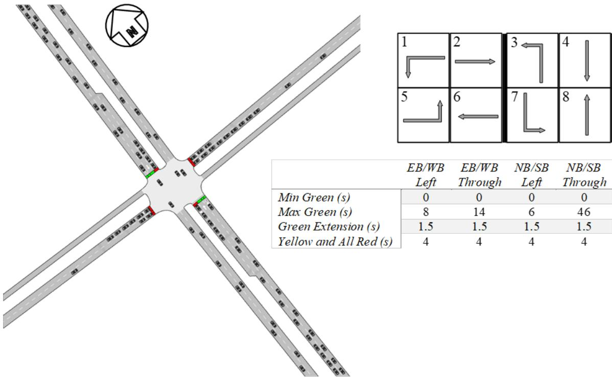
Figure I.2.1.6 Simulated intersection and signal control parameters
