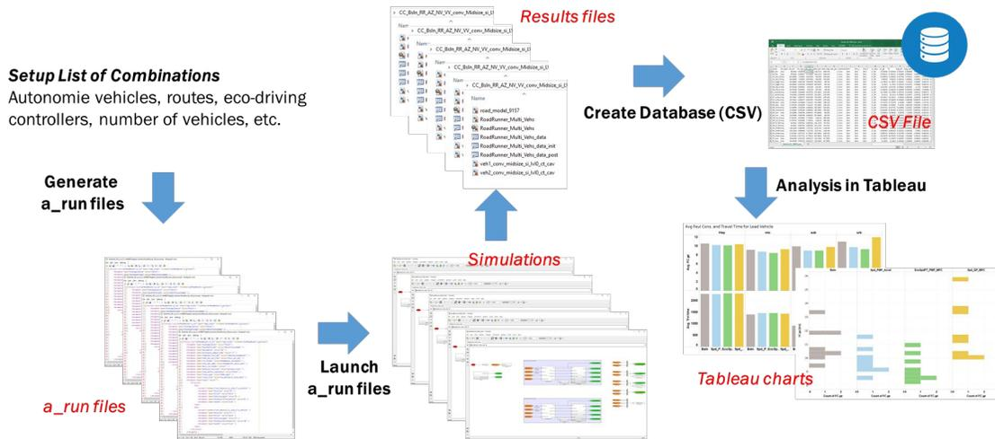
Figure I.6.2.3 Large-scale RoadRunner simulation workflow
