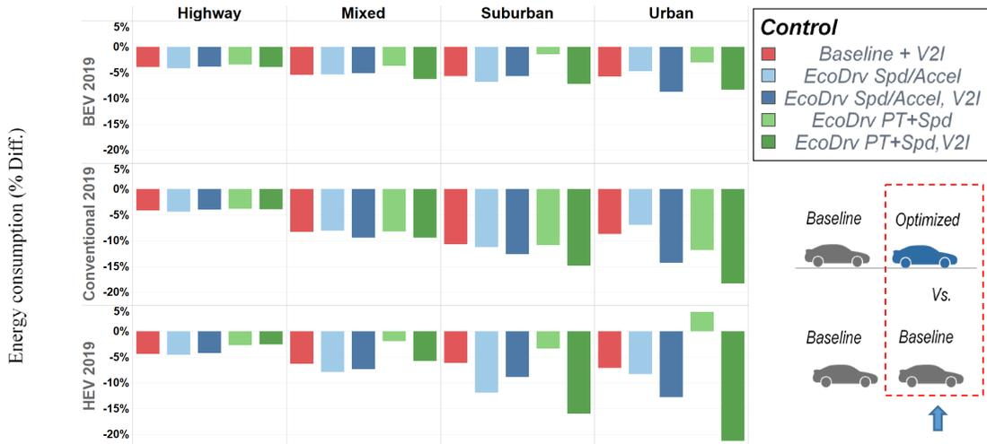
Figure I.2.3.5: Energy consumption savings relative to baseline control for a vehicle in lead position, with current powertrain technology, for various powertrains
