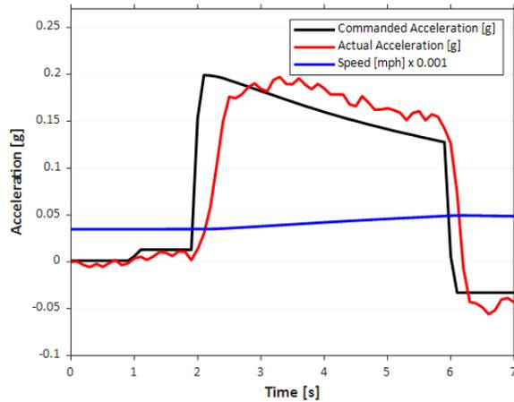
Figure I.2.7.11 Powertrain response to accelerator pedal override on 2014 Honda Accord
