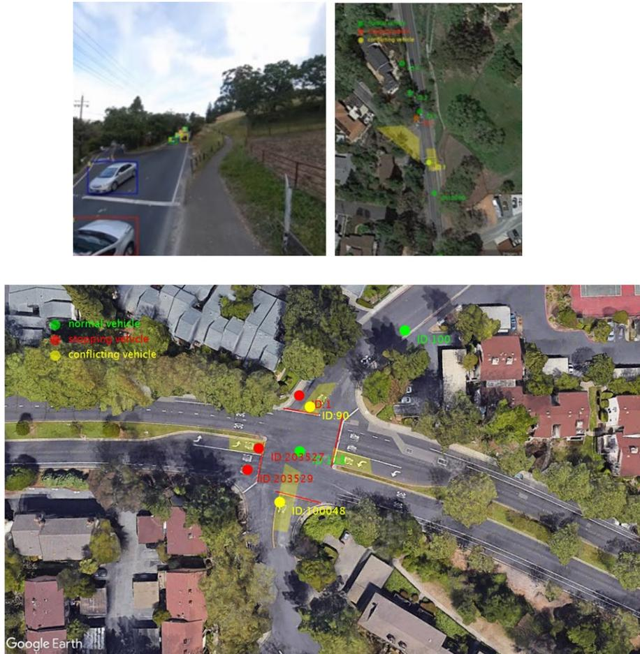
Figure I.2.8.2 Vehicle detections at a stop sign controlled intersection in Pleasant Hill, California
