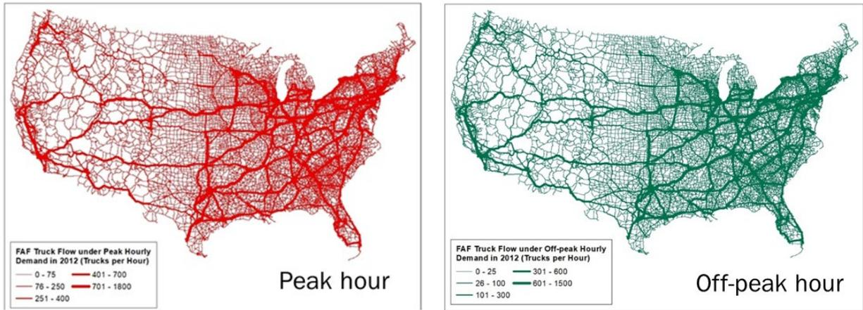
Figure I.4.1.5 Results of truck network assignment and temporal disaggregation
