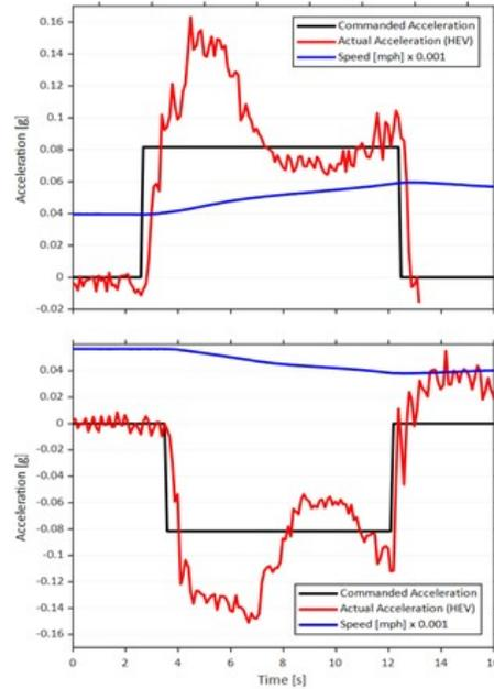
Figure I.2.7.3 Powertrain response to ACC acceleration override for 2017 Prius Prime
