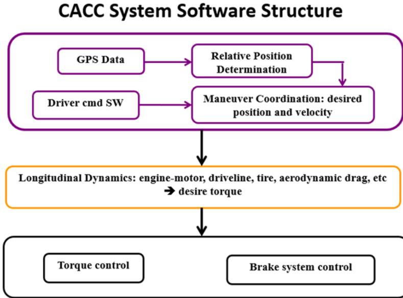
Figure I.2.7.1 Overall CACC System Structure for vehicles with all types of powertrains
