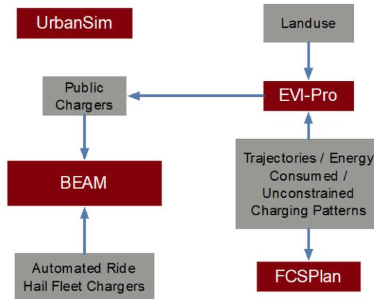
Figure I.6.4.2 Modeling workflow between BEAM, EVI-Pro, and FCSPan (Fast Charging Station Plan) to site charging infrastructure for BEAM simulations.
