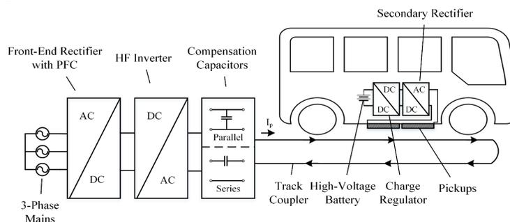
Figure I.1.3.1 Block diagram of a typical track-based dynamic wireless power transfer system.
