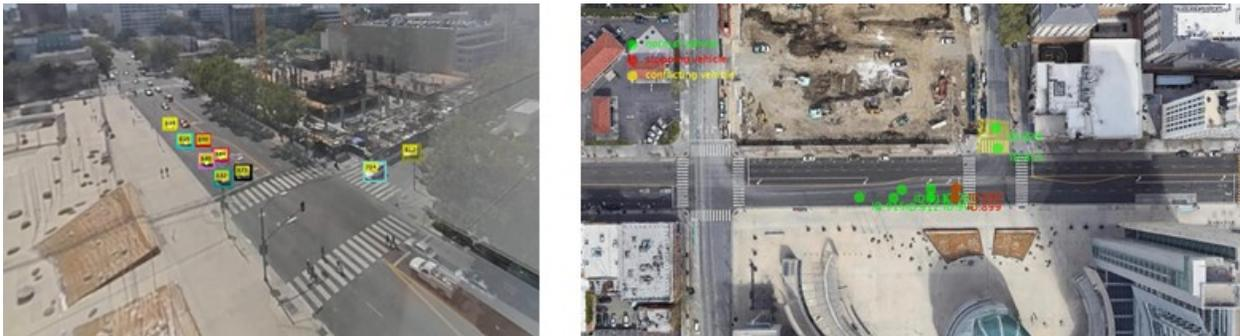
Figure I.2.8.1 Vehicle detections at Santa Clara St./4<sup>th</sup> St. in San Jose, California
