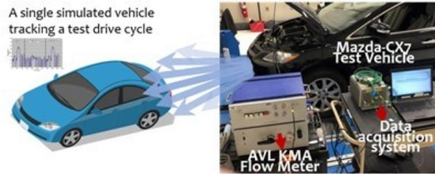
Figure III.1.2.3 The chassis dynamometer VIL setup.
