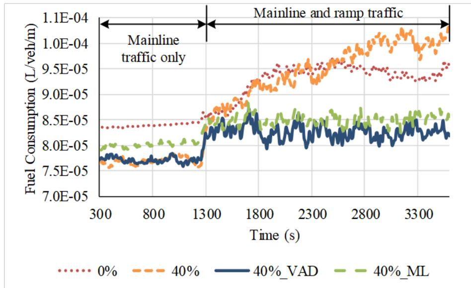
Figure I.2.1.5 Temporal and spatial patterns of the vehicle fuel consumption rate for the 40% CACC case
