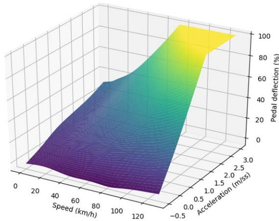
Figure I.2.7.8 Accelerator pedal map for 2013 Ford Taurus
