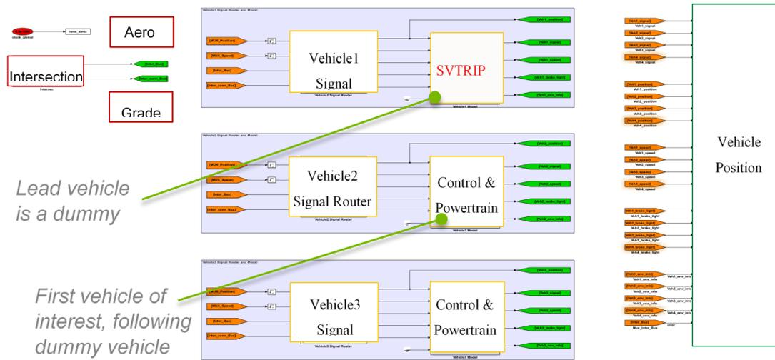
Figure I.6.3.2 Simulink diagram of a RoadRunner scenario with dummy lead SVTRIP vehicle
