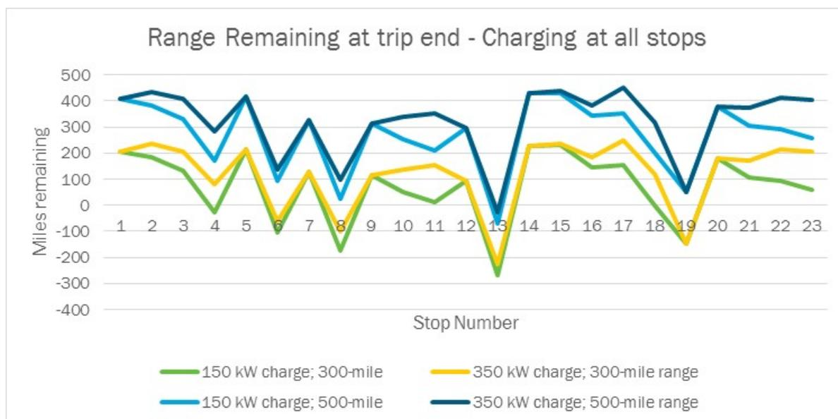
Figure I.1.4.7 Range remaining at each stop if charging is available at each stop
