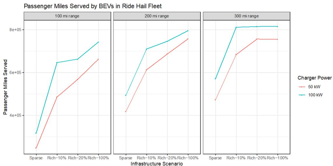
Figure I.1.2.10 Passenger miles served by EVs in ride-hailing fleet by infrastructure scenario (x-axis), vehicle range scenario (panel), and charger power scenario (trend color)
