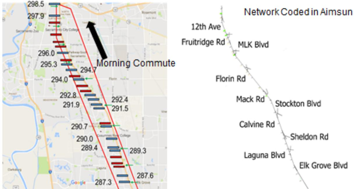
Figure I.6.1.4 Microscopic traffic simulation in Aimsun. Left: the scope of the freeway corridor with location of detector stations from PeMS; Right: the Aimsun network model
