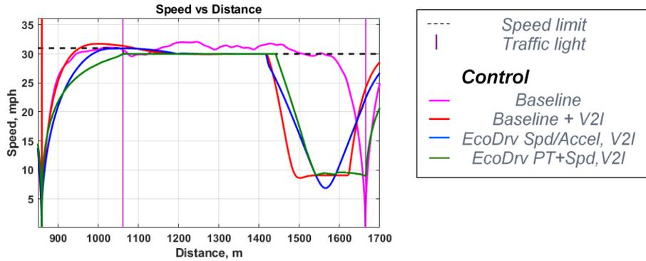
Figure I.2.3.4 Speed traces for a BEV with different control strategies
