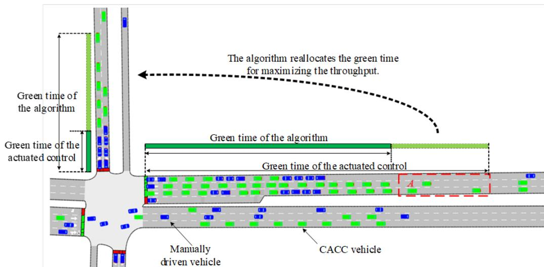
Figure I.2.6.2 Comparison of the proposed algorithm and actuated control
