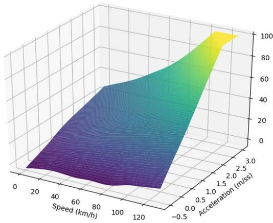
Figure I.2.7.10 Accelerator pedal map for 2014 Honda Accord
