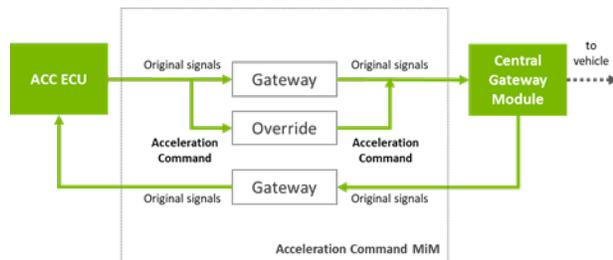
Figure I.2.7.14 ACC acceleration command override MiM diagram
