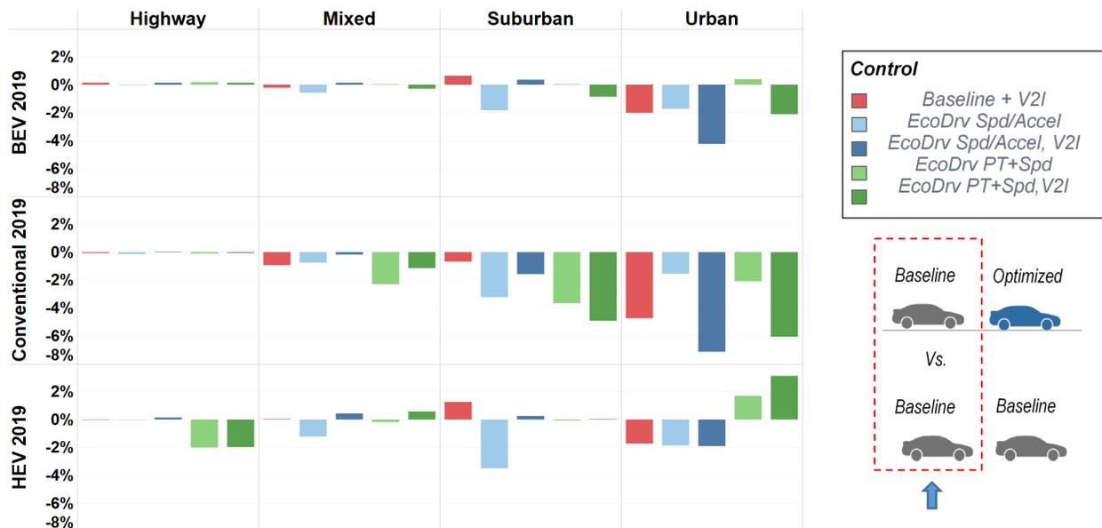
Figure I.2.3.8 Energy consumption of following baseline vehicle (lead: control versus baseline) with current technology and various powertrains
