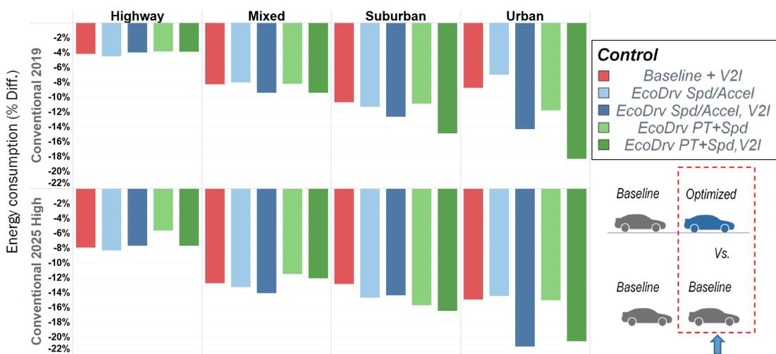
Figure I.2.3.6 Energy consumption savings for lead vehicle, conventional, current versus future technologies
