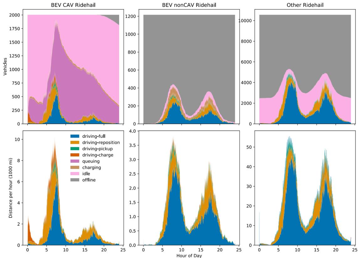
Figure I.1.2.11 Distribution of the ride-hailing fleet into operating states over the 24-hour simulation period for scenario with 100-mile range EVs and sparse, 50-kW charging infrastructure. Horizontal panels separate vehicle types and vertical panels separate time spent by each vehicle (top) and distance traveled by all vehicles (bottom).
