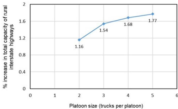
Figure I.4.1.8 Impact of platoon size on rural interstate highway capacity
