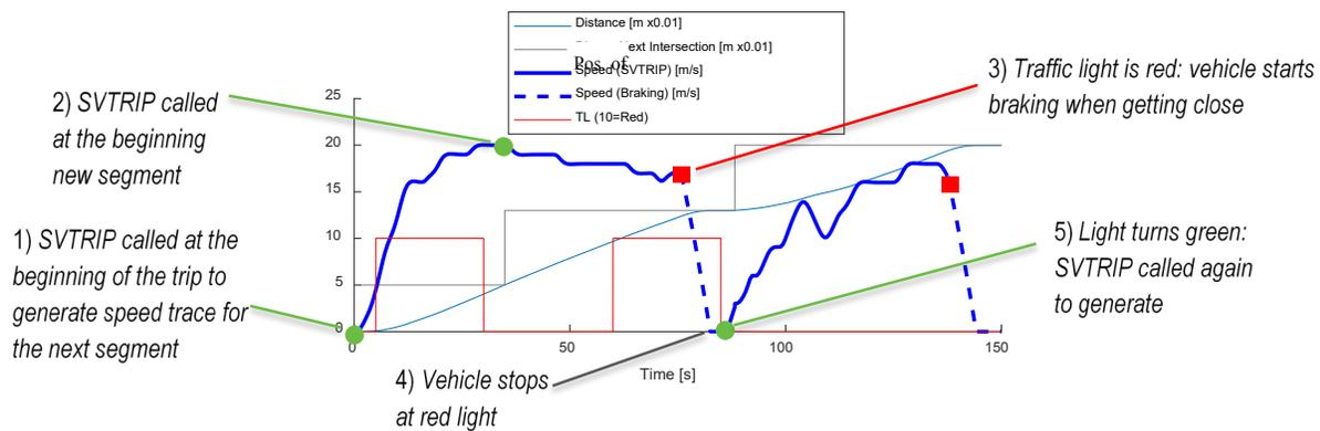
Figure I.6.3.5 Speed of dummy SVTRIP vehicle called within RoadRunner
