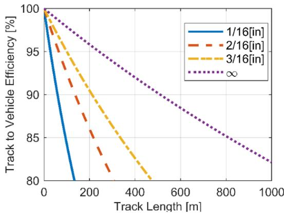
Figure I.1.3.2 Efficiency analysis of track-based DWPT system with respect to the track length.
