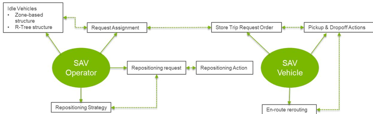
Figure I.2.2.1 Flowchart for SAV fleet operation in POLARIS
