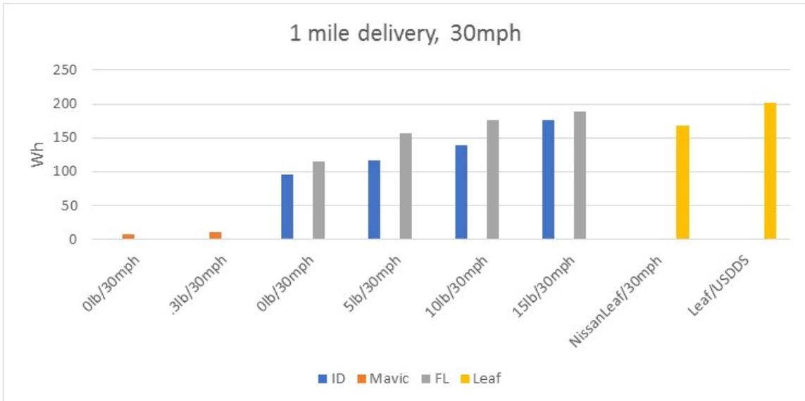
Figure I.4.2.1 Energy Estimates from one-mile delivery tests (INL)
