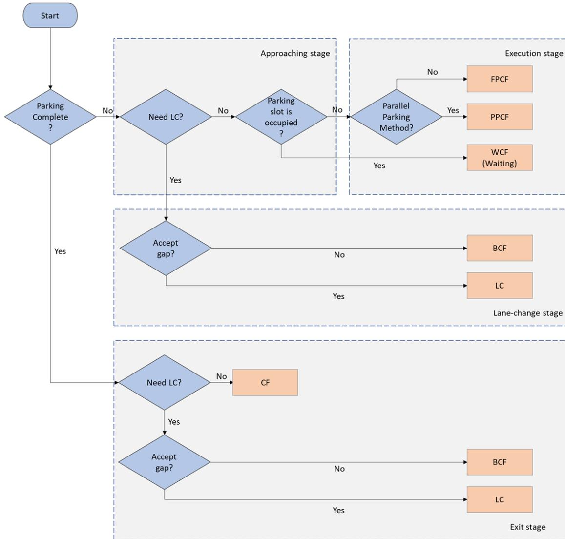
Figure I.6.1.2 Parking Maneuver Algorithm
