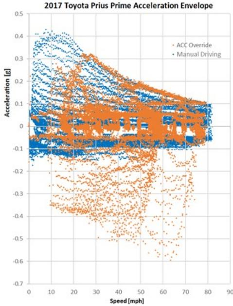
Figure I.2.7.2 ACC override acceleration envelope for 2017 Prius Prime
