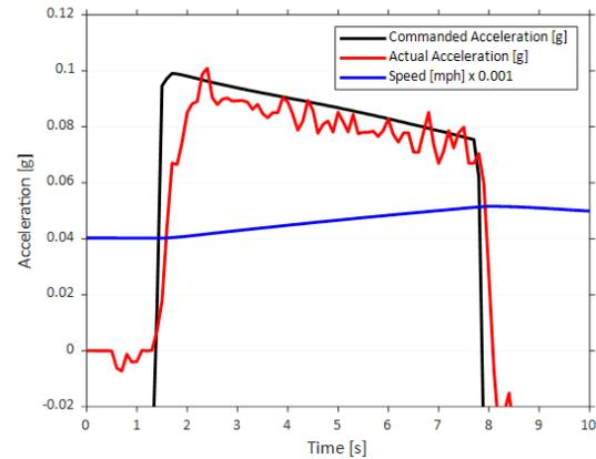
Figure I.2.7.5 Powertrain response to accelerator pedal override on 2017 Toyota Prius Prime
