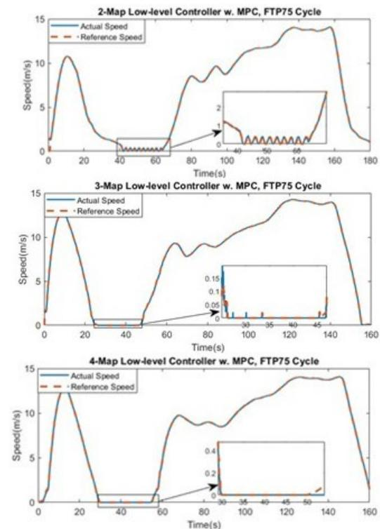
Figure III.1.2.9 Low-level speed controller performance comparison at low speed range
