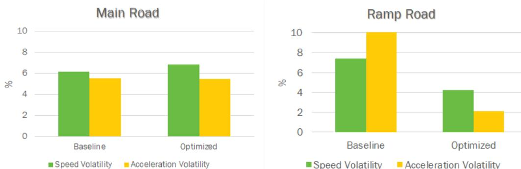
Figure I.2.4.10 Speed and acceleration volatilities in the main road, and ramp
