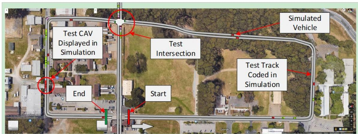
Figure I.2.6.5 Layout of the test track
