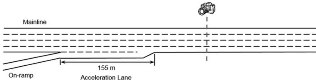
Figure I.2.1.2 Multilane freeway merge section
