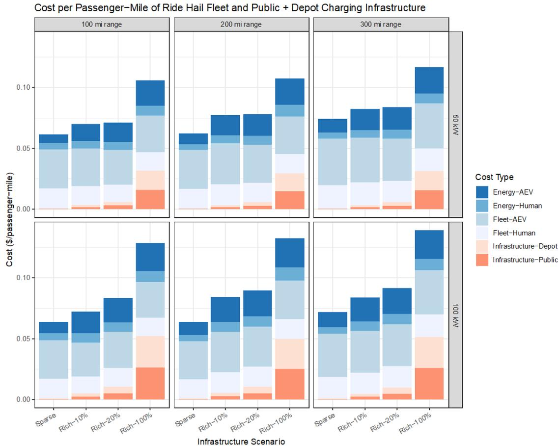
Figure I.1.2.13 Cost per passenger mile for the EVs in the ride-hailing fleet (both human-driven and AEVs), for both networks of fast charging infrastructure (both public and depot), and for the electricity and demand chargers necessary to supply the fleet with energy. The passenger miles traveled are only those that occur in EVs. The range scenarios vary with the columns of the panels, the power capacity scenarios vary with the rows, and the infrastructure scenarios vary across the x-axis.
