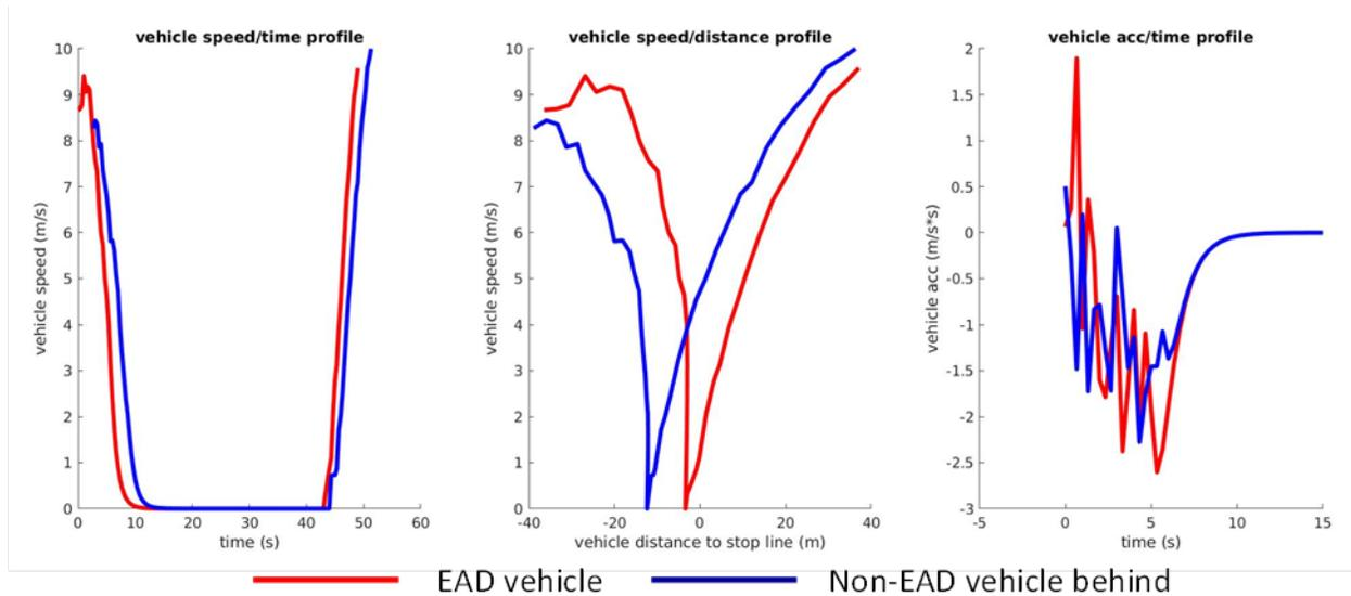
Figure I.2.8.5 EAD Case I: a no-EAD vehicle follows the EAD vehicle
