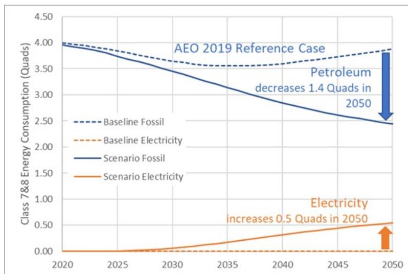
Figure I.4.1.10 Projected petroleum savings potential due to class 7&8 truck electrification
