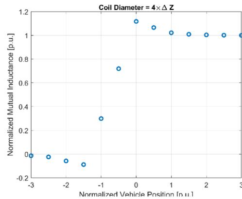
Figure I.1.3.3 Variation of the track-to-vehicle mutual inductance with respect to vehicle position.
