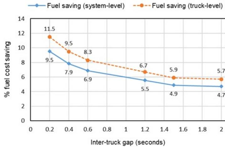
Figure I.4.1.7 Impact of inter-truck gap on fuel cost savings
