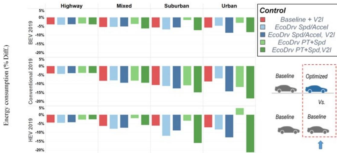
Figure 3 Energy Consumption Savings Relative to Baseline for Lead Vehicle
