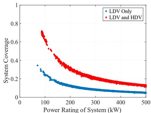
Figure I.1.3.4 Pareto solutions from the optimization model for two different cases (LDV only and LDV and HDV together).
