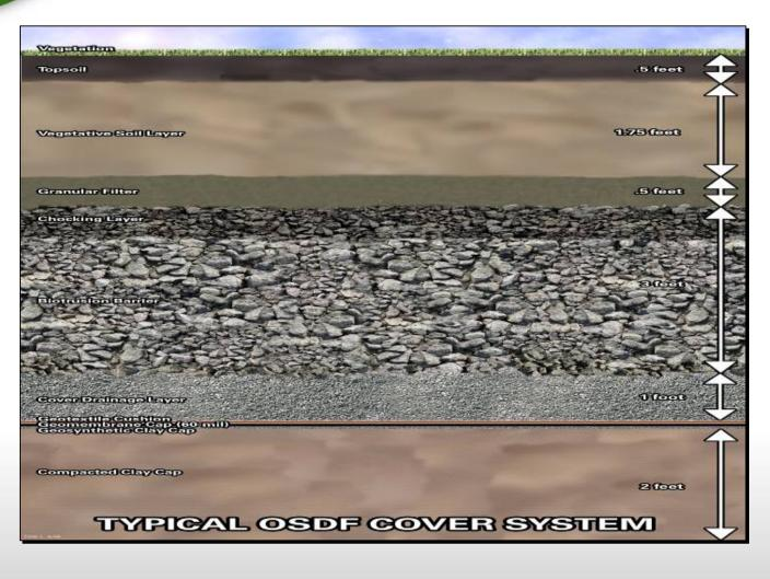
The On-Site Disposal Facility's engineered cover system.
