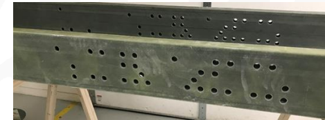
Box Section Frame Rails With Suspension Mounting Holes
