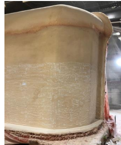
Mold Material Added To Trailer Front
