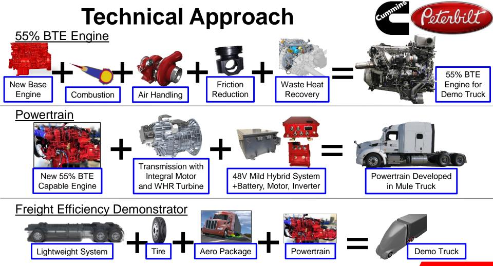
New Hardware: Engine & 55% BTE technology, transmission & 48V hybrid, axle, truck chassis, cab, aero, and tires.
