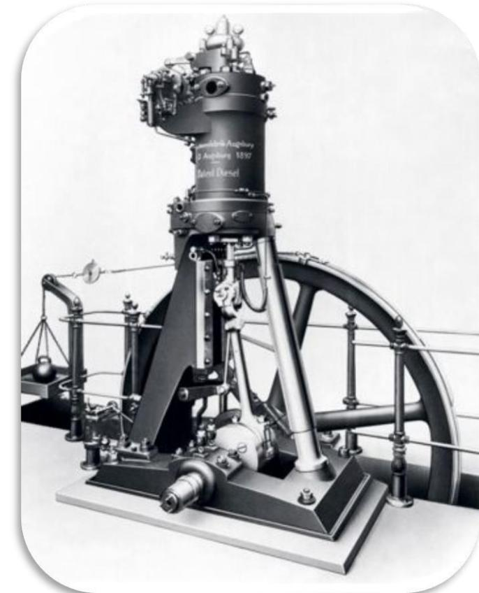
1 cylinder, four-stroke, water-cooled, air injection of fuel
