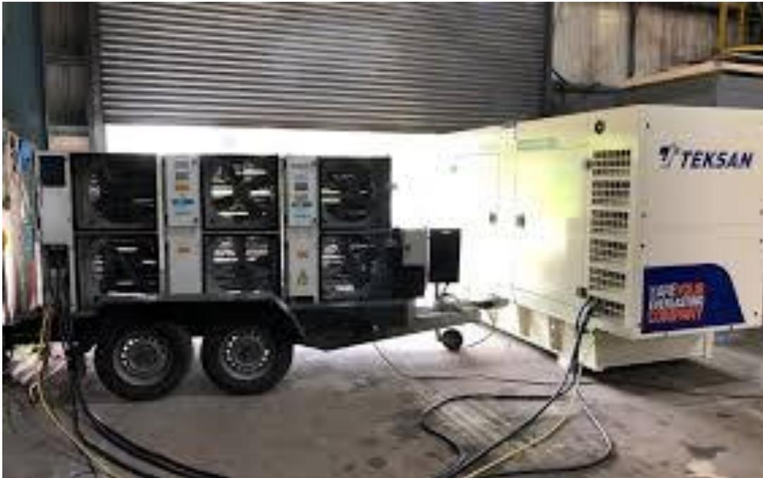
Standby generator load bank test
