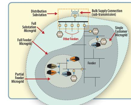
“Microgrids” can connect and disconnect from the main grid.
