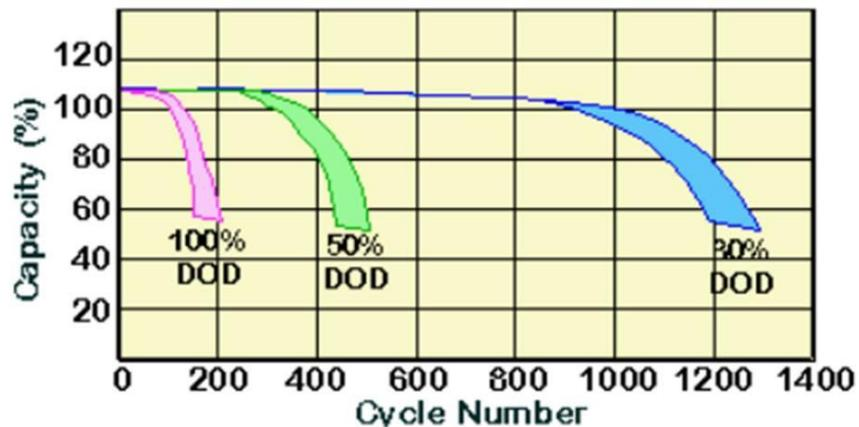
Battery cycle life depends on depth of discharge (DOD)
