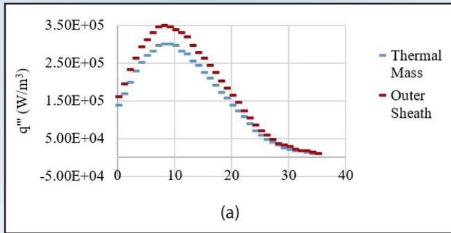
Figure 3. Energy deposition rate in the thermal mass and outer sheath of the OFBGT in the CIF.
