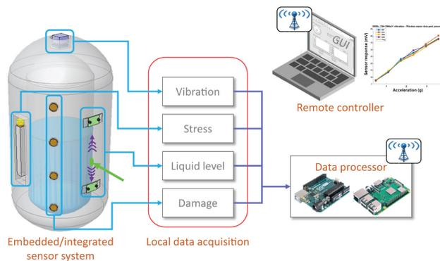
**Figure 1. Overview of HiTEIS with the wireless data communication.**
