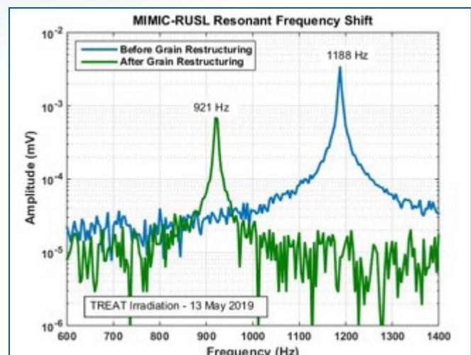
Figure 2. Resonant frequency before and after grain restructuring.
