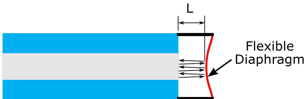
Figure 1. Diagram of a diaphragm-based extrinsic Fabry-Perot pressure sensor.
