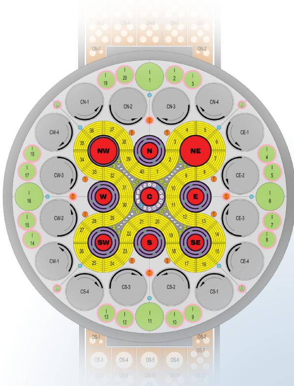
Figure 2. ATR core cross section with irradiation positions relevant to the FAS highlighted in red.
