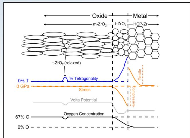
**Figure 3. Schematic summarizing the different parameters for each zirconia and zirconium phase.**
