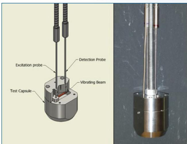
Figure 1. Section view of the test capsule showing the cantilever beam with excitation and detection probes (left), capsule prior to reactor test (right).
