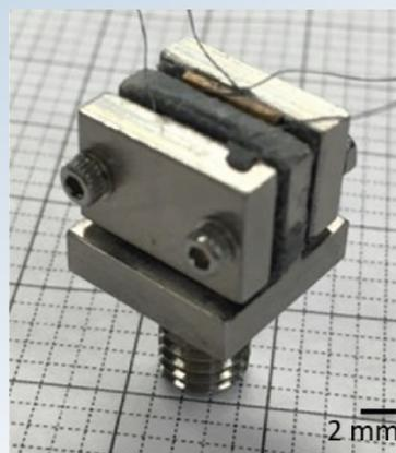
**Figure 2. Vibration sensor for NPP application [8].**
