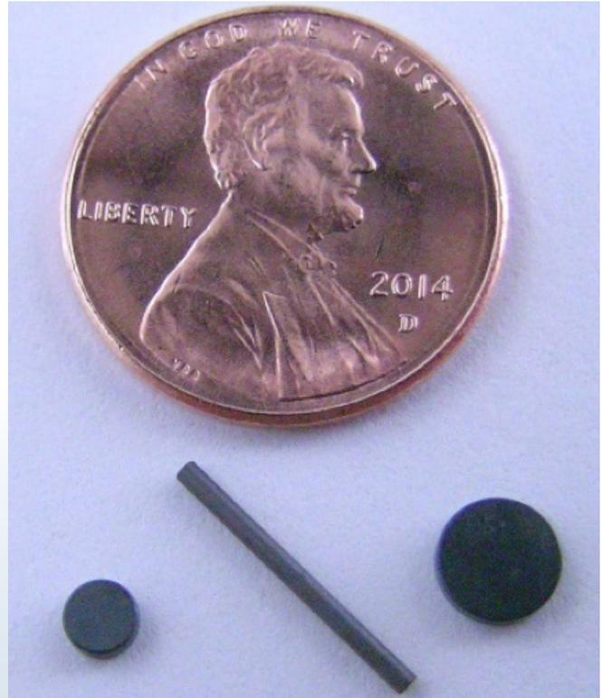
**Figure 1.** SiC temperature monitors available for use in irradiation testing include small rods and discs. Monitors photographed with U.S. cent for size perspective. [1]
