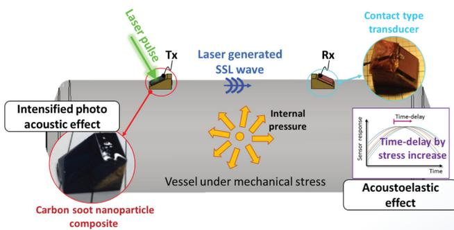
Figure 3. Laser assisted stress sensor [9].
