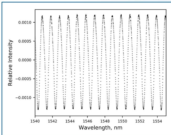
**Figure 2.** Measured interference spectrum from extrinsic Fabry Perot cavity.
