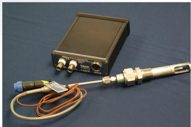
Figure 1. Sporian flow sensor with drive electronics.
