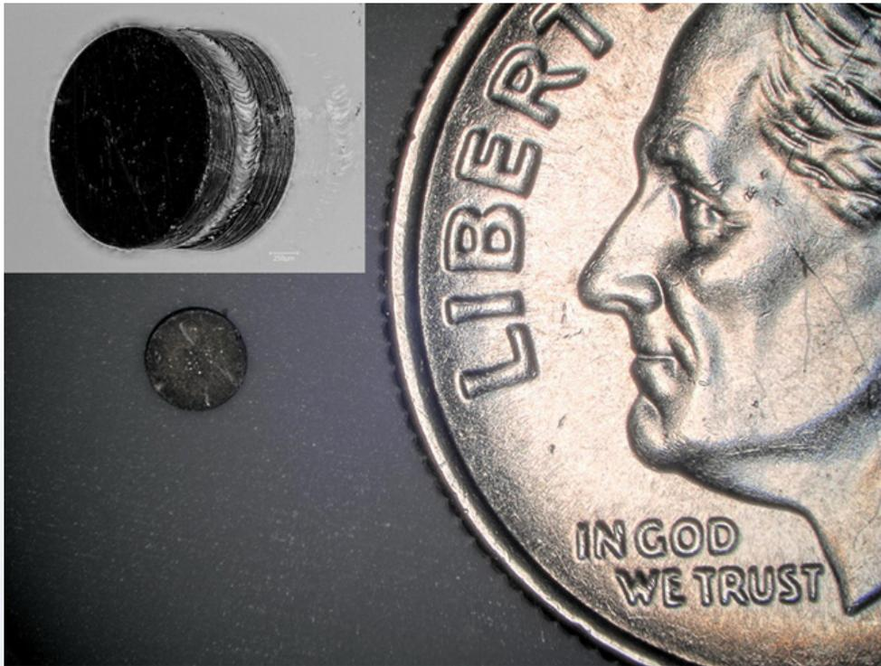
*Figure 2. 2-mm-diameter melt wire sensor chip alongside a dime. The inset shows clear view of laser welded chip.*
