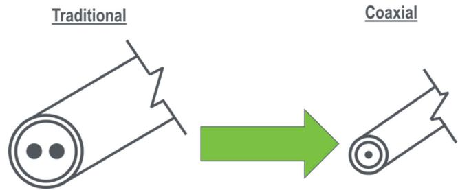
**Figure 2. Traditional HTIR-TC mineral insulated metal sheathed cabling versus the optimized “coaxial” cabling. The coaxial cable provides builds with longer lengths, smaller diameters, and more robust performance.**
