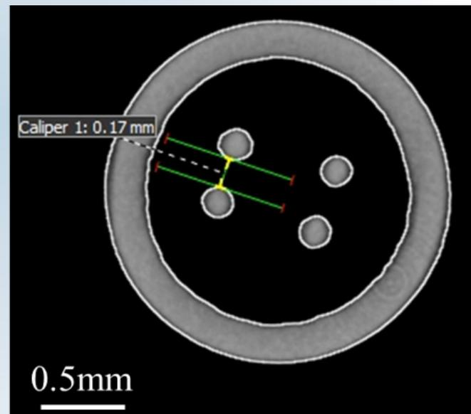
**Figure 1. Cross section of the sample and needle probe geometry.**
