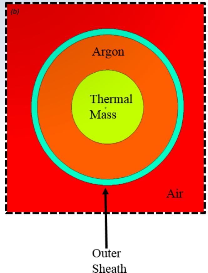
Figure 2. (a) Top-down view showing the simple OFBGT design within the CIF tube in the MCNP model of the OSURR. (b) Close-up view of the simple OFBGT geometry itself.
