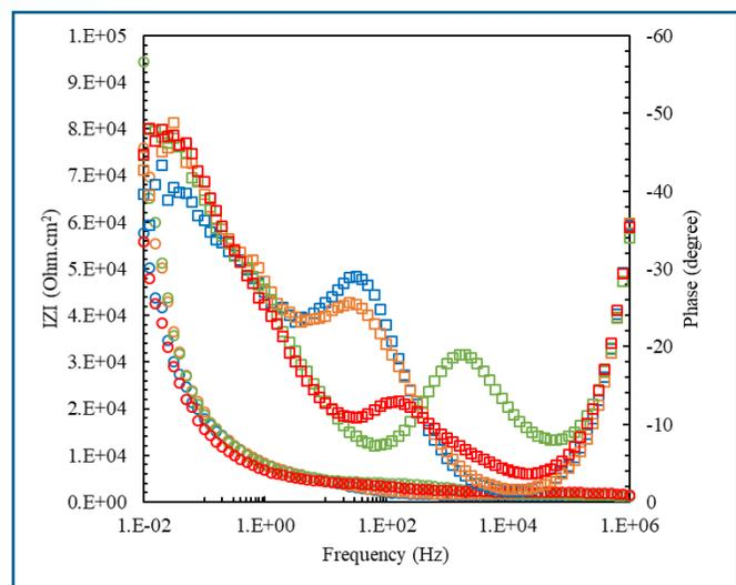
**Figure 1. Impedance spectra for sample Zr-4 as a function of immersion time: left for Nyquist and right for Bode plot.**
