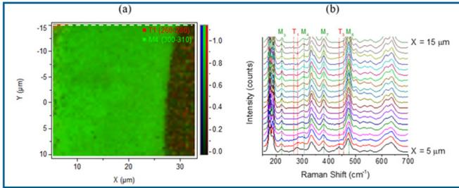
**Figure 2. Raman mapping for Zr alloy: (a) Co localized mixed intensity maps presenting tetragonal, T1 (red) and monoclinic, M4 (green) peaks. (b) Waterfall of Raman spectra near the metal/oxide interface, corresponding to the dotted line in the mixed intensity map.**
