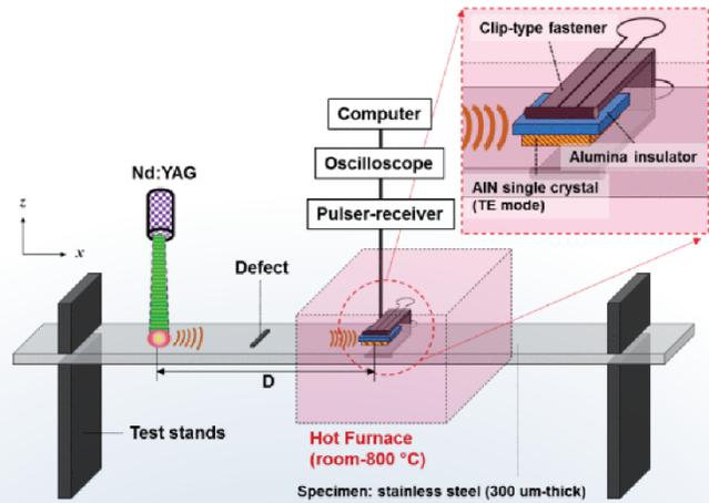
Figure 5. Laser-assisted HT damage detector [10].
