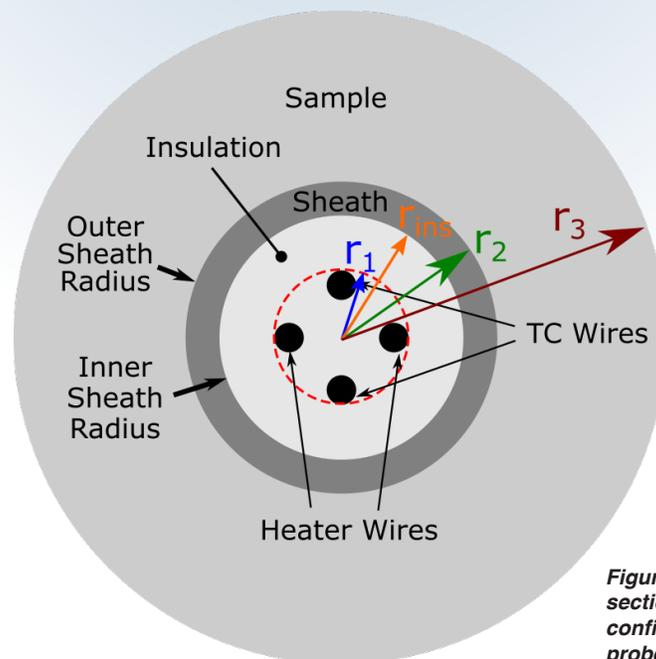
**Figure 2. Diagram of the cross section of the experimental configuration showing the needle probe internals at the center.**
