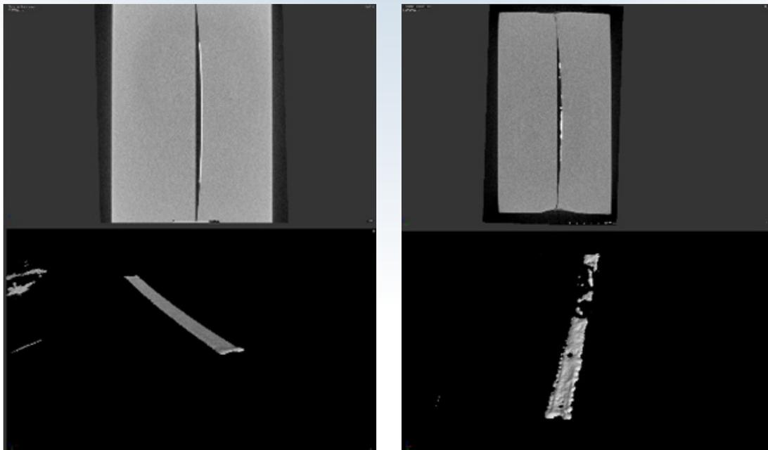
**Figure 3.** X-ray CT scan of the melt wires (left) before heating, and (right) after heating to 1000°C inside a furnace. The upper images show a cross section of the entire chip, and the lower images show just the meltwire.
