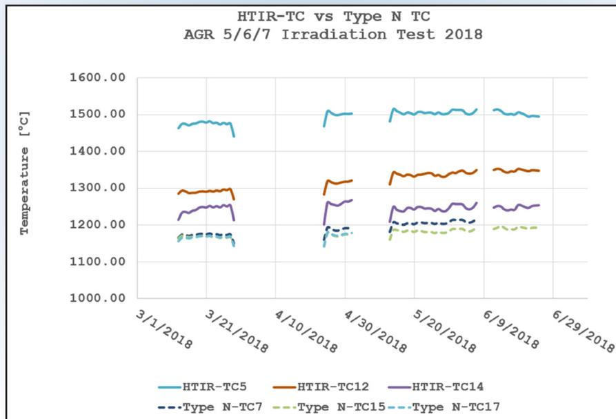
**Figure 1.** A small window of data for the AGR 5/6/7 results of HTIR-TCs and Type N TCs; showing the HTIR-TCs outlasted and outperformed the Type N TCs in near vicinity.
