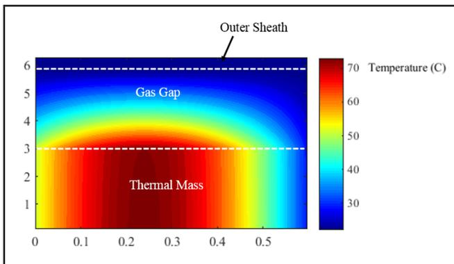
Figure 4. Temperature distribution in the OFBGT in the CIF of the OSURR.
