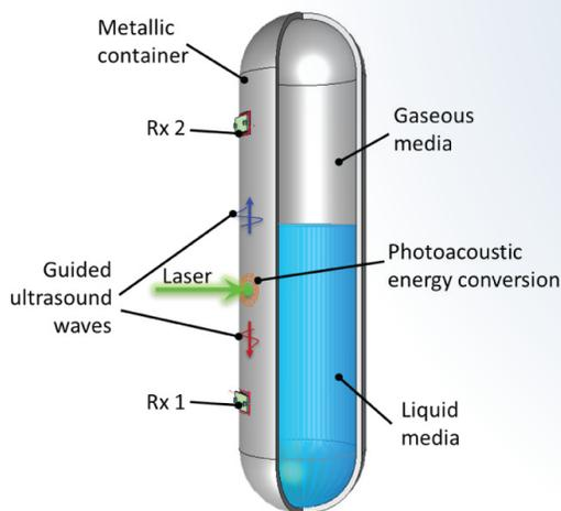
Figure 4. Laser-assisted HT liquid level sensor.
