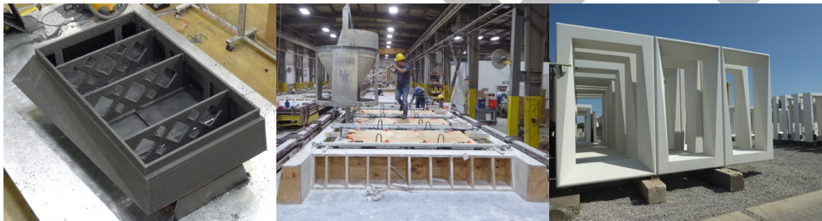
Figure 4-1: Additive manufacturing has been demonstrated successfully for precast concrete forms of building facades. Avenues to employ advanced manufacturing techniques, such as additive manufacturing, for energy-efficient building envelope components merit additional investigation. (ORNL/Diana Hun)
