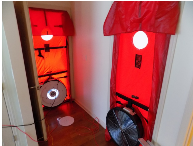
Figure 2-7: Guarded blower door tests, shown here set up in a single-family home, are similar to standard blower door tests, but use additional fans to isolate specific sections of a building's facade.
