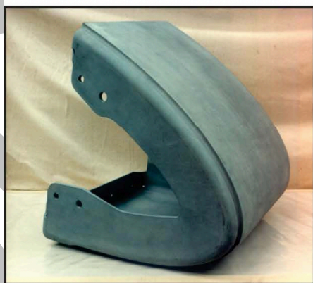
Figure 3-7: Reinforced carbon-carbon is a graphite-reinforced carbon composite matrix with thermal anisotropy used for the nose cap and wing leading edges of the Space Shuttle Orbiter. [44]
