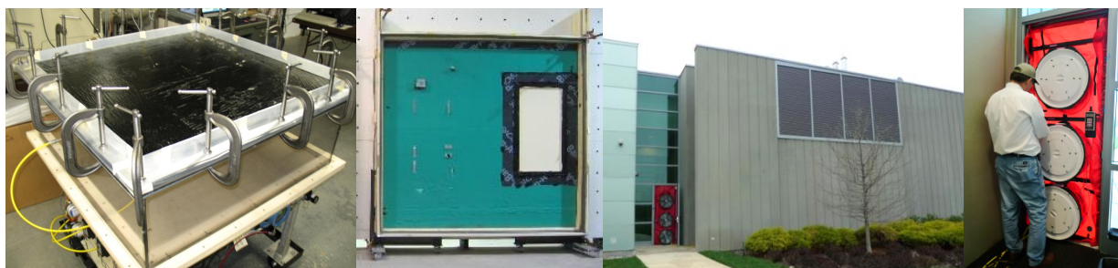
Figure 2-4: (a) Experimental setup to measure the air permeability of a 1-m by 1-m air barrier material in accordance with ASTM E2178; (b) Experimental setup to measure the air leakage rate of a 2.4-m by 2.4-m air barrier assembly in accordance with ASTM E2357; (c and d) Experimental setup to measure the air leakage rate of a building envelope in accordance with ASTM E779.
