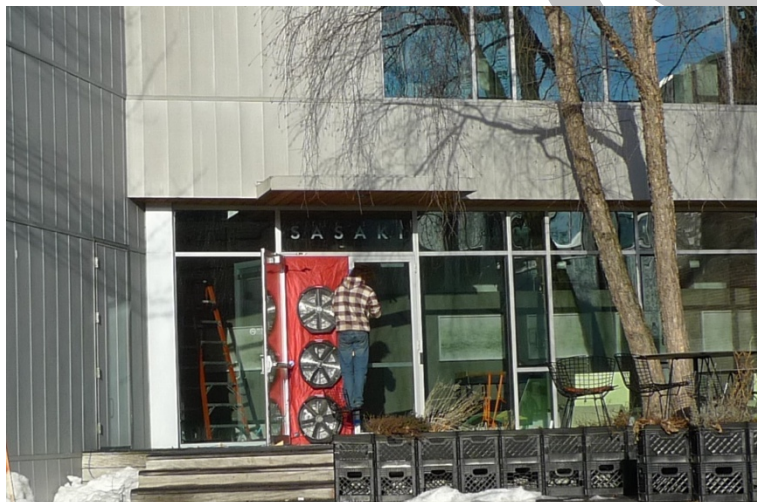
Figure 2-8: Blower door tests for commercial buildings can require much more equipment, which adds significantly to the setup and teardown time, as well as the complexity of performing the test itself.
