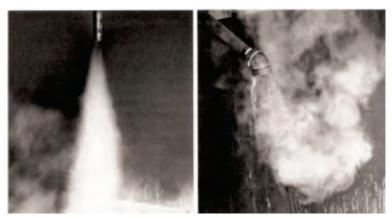
Figure 9.3.7. Live steam (left) versus flash steam (right)
