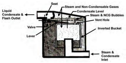
Figure 9.3.1. Inverted bucket steam trap
