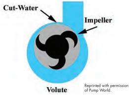
Figure 9.9.4. Centrifugal pump.
