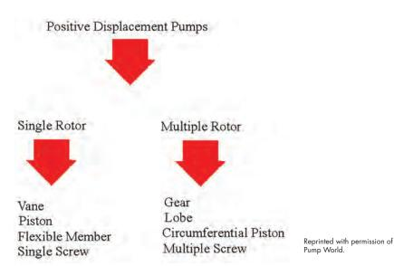
Figure 9.9.3. Positive displacement pumps.
