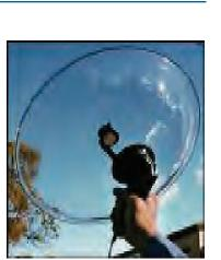
Parabolic dish used with ultrasonic detector greatly extends detection range abilities.
