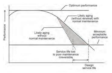
Figure 2.4.1. Effect of adequate and timely maintenance and repairs on the service life of a building (National Research Council 1998).
