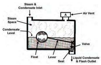
Figure 9.3.4. Float and thermostatic steam trap
