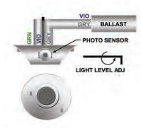
Figure 9.12.3. Photosensor and fluorescent dimming ballast for continuous daylight dimming.
