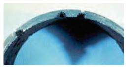
**Figure 9.2.10**. Feed-water pipe – oxygen pitting
