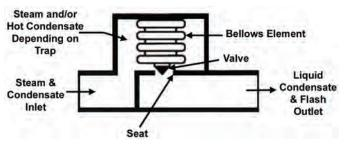
Figure 9.3.3. Bellows steam trap
