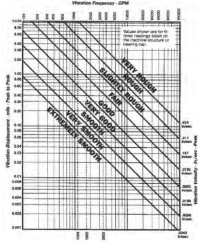
Figure 6.5.1. Vibration severity chart
