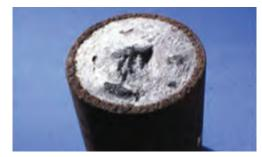
Figure 9.2.8. Boiler tube - scale deposit
