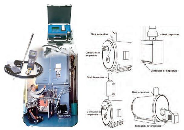
Figure 9.2.6. Combustion analyzer
