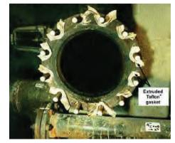
Figure 9.3.8. Failed gasket on blind flange
