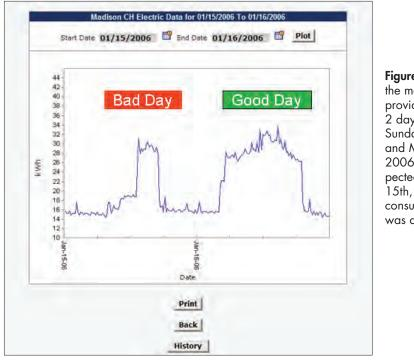
Figure 8.9.3. Data from the monitoring device provides a comparison of 2 days of electricity use for Sunday, January 15, 2006, and Monday, January 16, 2006. Figure shows unexpected off-hour usage on the 15th, while electricity consumption on the 16th was as expected.
