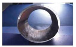
**Figure 9.2.13**. Condensate pipe – acidic corrosion
