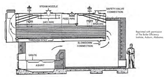
Figure 9.2.1. Horizontal return fire-tube boiler (hot gases pass through tube submerged in water).
