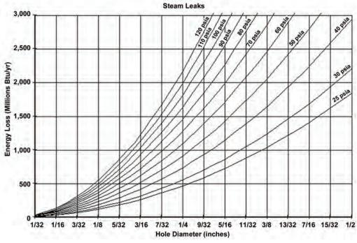
Figure 9.3.6. Energy loss from leaking steam traps.
