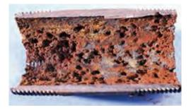
**Figure 9.2.12**. Condensate pipe – oxygen pitting
