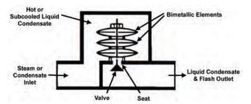
Figure 9.3.2. Bimetallic steam trap
