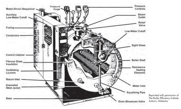
Figure 9.2.3. Electric boiler
