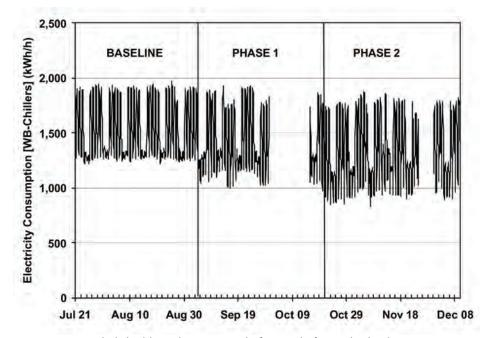
**Figure 7.9.1**. Whole-building electricity use before and after night shutdown program. Data gaps were periods when data were not available. Average nightime savings is 350 kW (1,250 kW – 900 kW).
