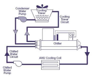
Figure 9.4.1. Typical chiller plant
