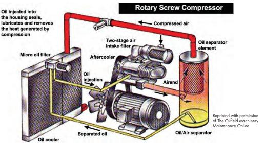
Figure 9.11.1. Rotary screw compressor
