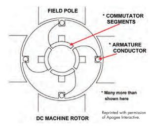
Figure 9.10.3. Parts of a direct current motor
