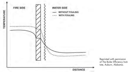
Figure 9.2.5. Effect of fouling on water side
