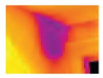
**Figure 6.2.2**. Internal house wall. Note dark area indicating cooler temperatures because of heat loss.
