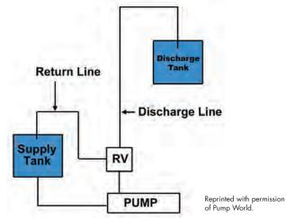
Figure 9.9.5. Schematic of pump and relief valve.
