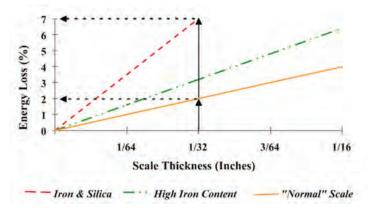
Figure 9.2.14. Boiler energy losses versus scale thickness
