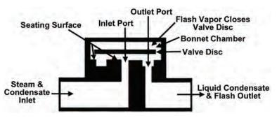
Figure 9.3.5. Disc steam trap
