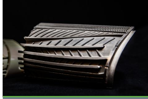
This project explores the use of advanced airfoil materials and designs as well as additive manufacturing approaches to increase system efficiency of gas turbines with less than 20 MW capacity. *Image courtesy of National Energy Technology Laboratory*
