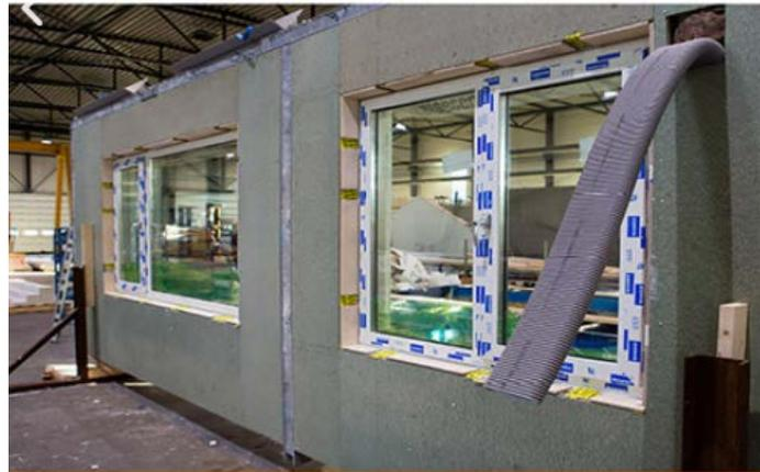
**Figure 10. Ducting integrated into Renolution facade panel**
