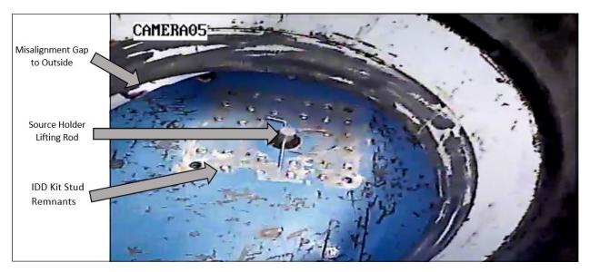
Figure 10: Image of Irradiator (blue) Beneath the MHC
