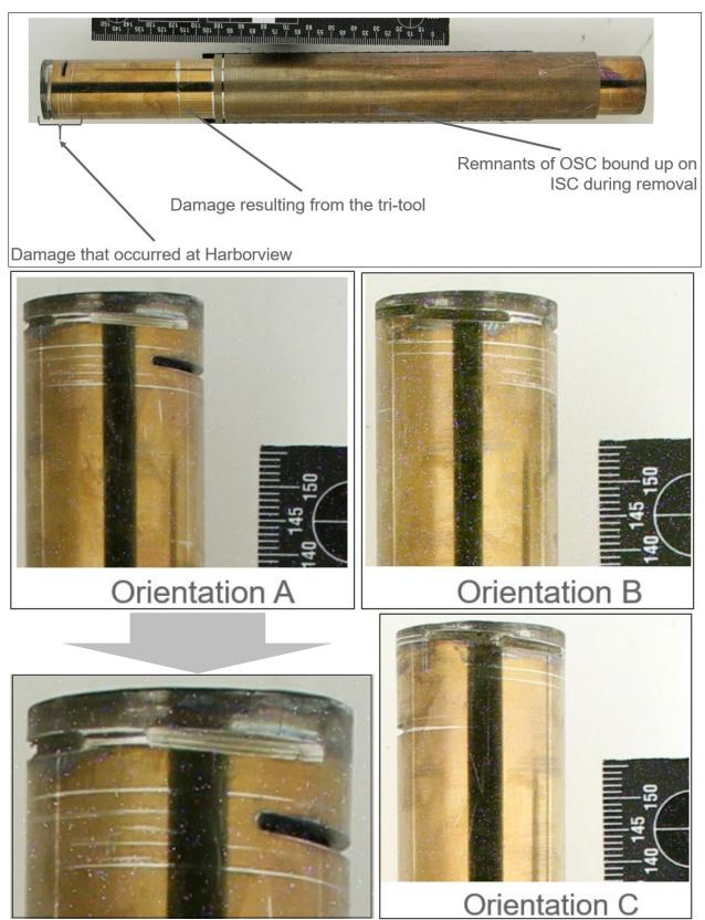
Figure 21: Damage to Cesium-137 Inner Source Capsule (Forensic images – Close ups show damage during source recovery operations.) (OSC: Outer Source Capsule; ISC: Inner Source Capsule)
