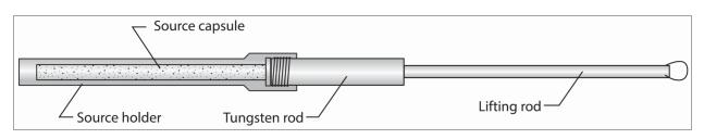
Figure 4: Notional Diagram of Source Holder
