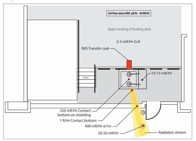
Figure 11: Radiation Fields During Source Removal Operation
