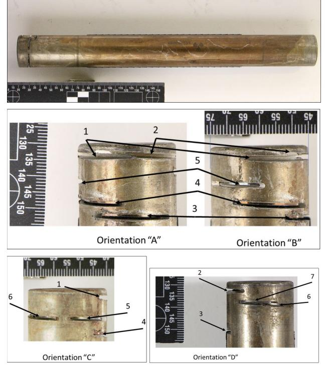
Figure 20: Damage to Cesium-137 Outer Source Capsule (Forensic images – counterclockwise rotation views.) (Numbers are references to identify the cuts into the outer source capsule)
