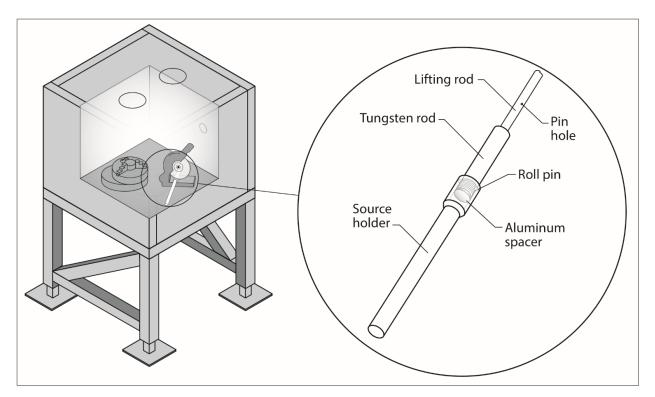
Figure 6: Mobile Hot Cell and Source Holder
