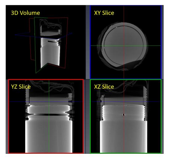
Figure 17: Tomographic Image of the Tungsten Rod
