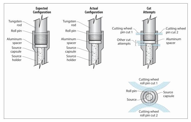
Figure 14: Notional Drawings of Source Holder Configuration
