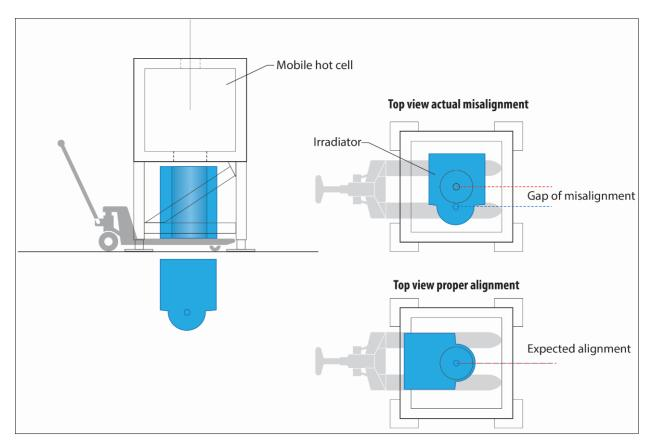
Figure 9: Notional Drawing of Irradiator (blue) Alignment Beneath the MHC
