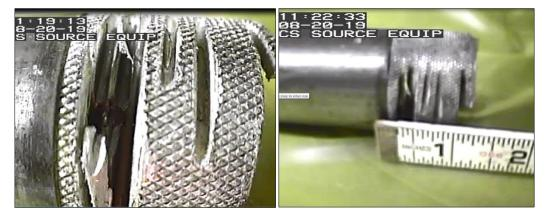
Figure 16: Cuts in the Vicinity of the Roll Pin – View 1 (left) and View 2 (right)
