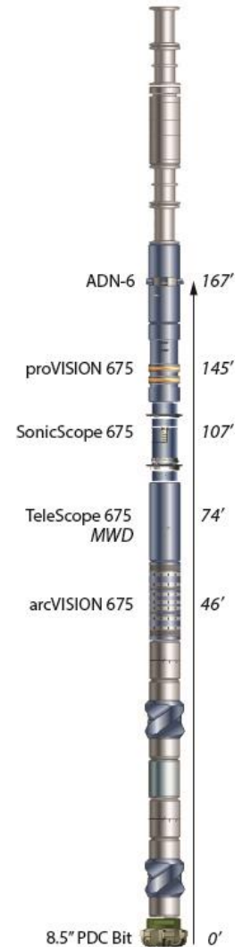
Bottom-hole assembly for main hole (from Schlumberger)
