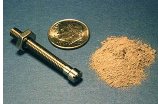
A titanium bolt and the corresponding amount of titanium powder necessary to create it.
