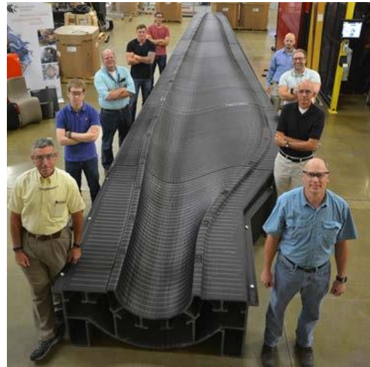
The ORNL Manufacturing Demonstration Facility Team next to a 3D printed wind turbine blade mold.
