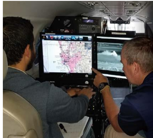
GA-ASI Field Engineers testing the new Claw interface for the Lynx radar
