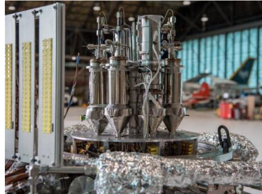
NASA's "Kilopower Reactor Using Stirling Technology" system, affectionately abbreviated "KRUSTY."
