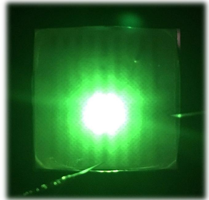
*Green OLED on Diffuse Reflector Substrate*
