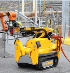
The KUKA robotic arm attached to the BROKK 100 robotic base (left) is a specialized combination of two commercially available robotic devices that were modified by SRR to work as one robot for performing remote repair work in the liquid waste facilities. The robots were used to detect leak sites and perform repair work in the 3H Evaporator vessel.
