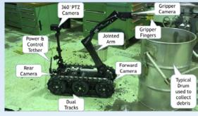
robot can use tools, such as a push broom and dust pan, to move and collect bulk volumes of glass. A similar crawler was used to inspect the sand filter at DWPF.
