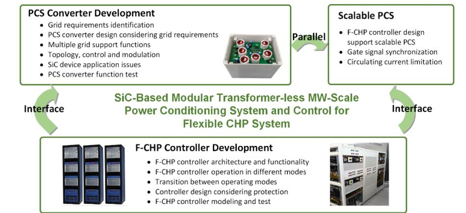
Summary diagram of the key project technologies being developed: The power conditioning system (PCS) converter, scalable PCS, and the flexible CHP (F-CHP) controller. *Graphic courtesy of the University of Tennessee, Knoxville*
