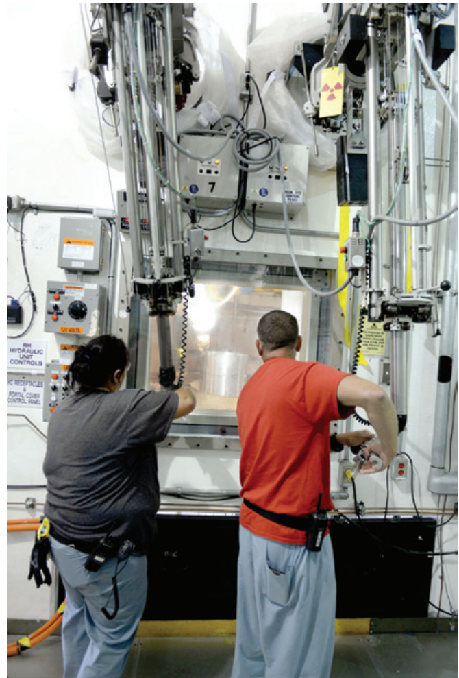
TWPC operators using manipulators to process highly radioactive transuranic waste inside the hot cell
