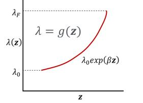
$\mathbf{z} = (z_1, ..., z_n)$  is the vector of *n* performance parameters measured for the component and g() is a function capturing component failure due to degradation
