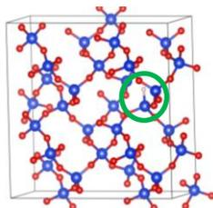
Modeling oxygen deficient centers (ODCs) and the effect of H dopant on refractive index
