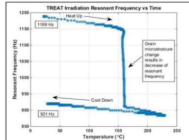
1st flexural mode resonance shift due to recrystallization
