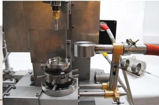
Halden equipment to instrument pre-irradiated fuel rods
