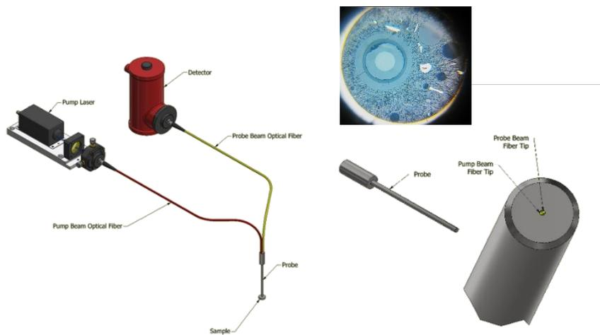
Fiber-optic based in-pile system
