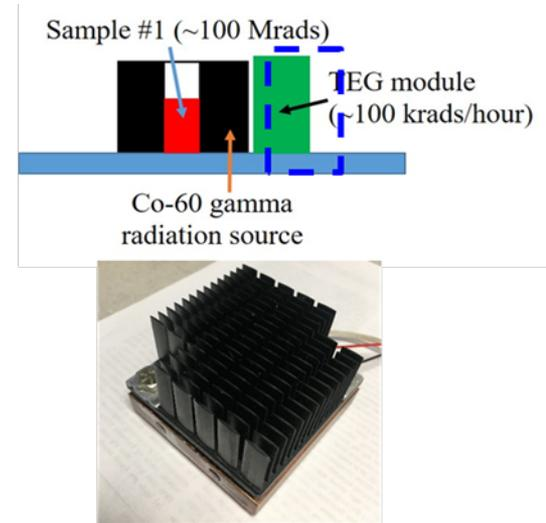
Experimental setup in the chamber
