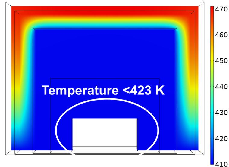
Temperature distribution in the shielding block
