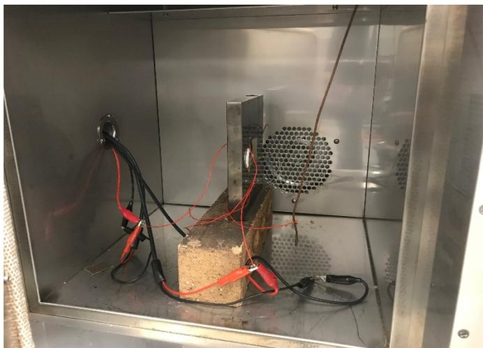
Through wall communication modulus in a oven.
