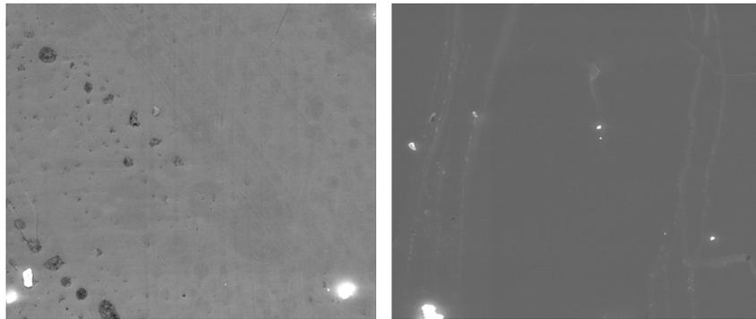
SEM images before and after test, 5000-time magnification.
