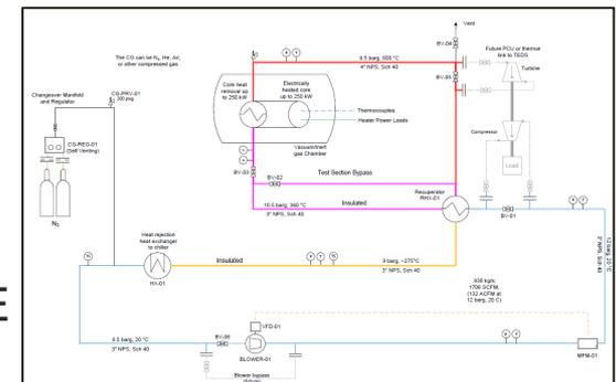
Preliminary Non-Nuclear Testbed Component Diagram
