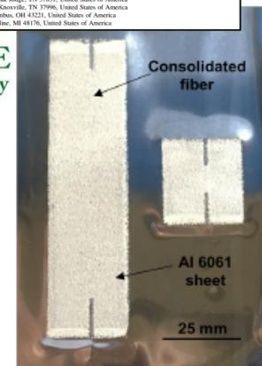
Embedded fiber sensors previously developed at ORNL
