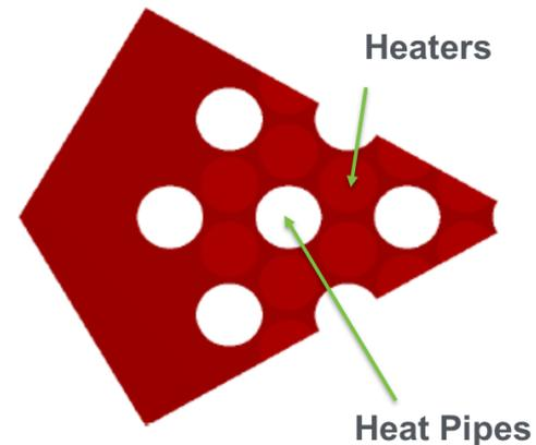
1/6th of test article showing heat pipe and heater location
