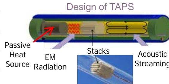
TAPS Prototype for In-sodium Test
