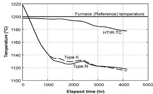
HTIR drift compared with type N, K
