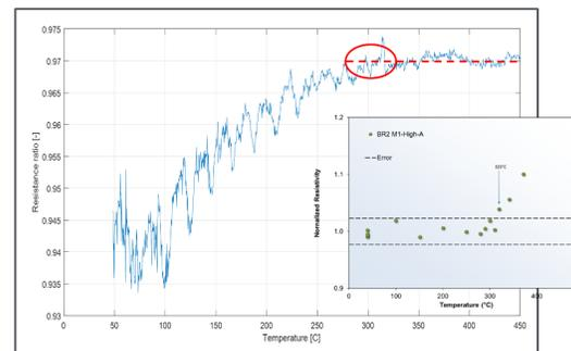
Continuous reading of SiC monitors in PIE after BR2 irradiation
