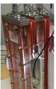
Series connection of electrolytic cells – biopolar stack configuration
