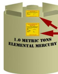
Figure 2: 1-MT Container Label Placement
