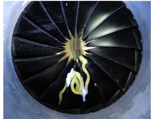
Self cleaning feature verified during water tunnel test
