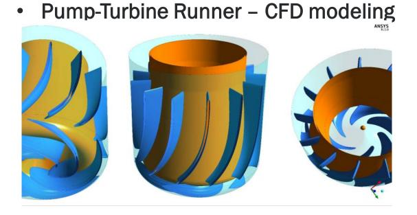
Hydraulic Best Efficiency: Pump Mode = 95.2% Turbine Mode = 94.5%
