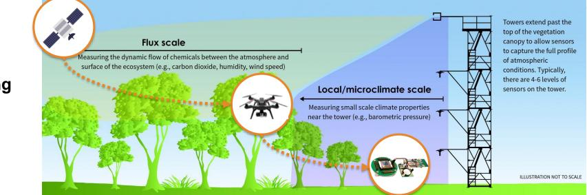
Aboveground monitoring of N<sub>2</sub>O, CO<sub>2</sub>, CH<sub>4</sub> flux
