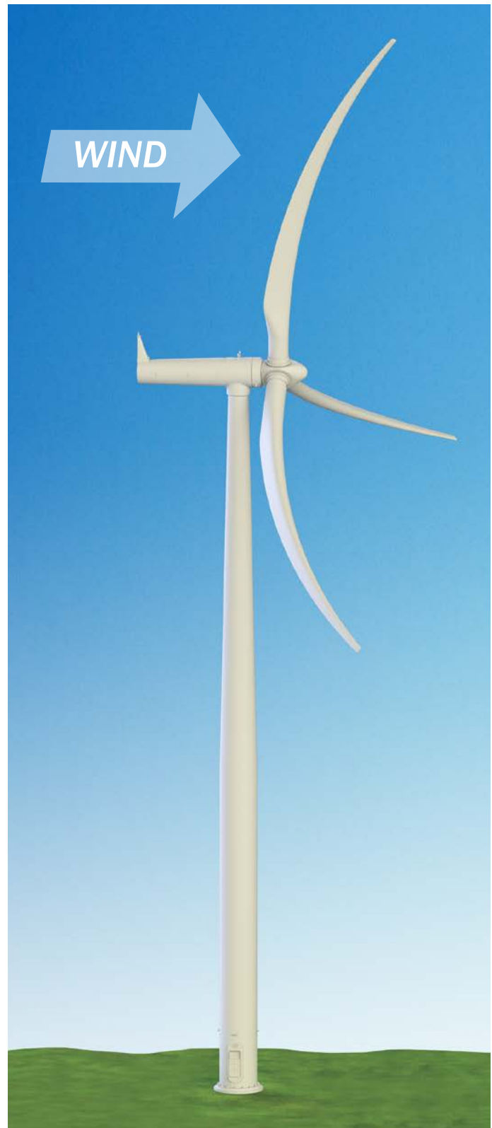
Downwind turbines like the one shown here could allow for taller turbines and longer blades because the wind pushes the blades away from the tower, enabling increased tower clearance. Graphic by NREL
