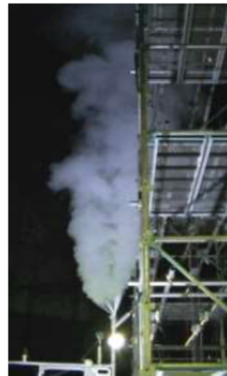
LH2 Leakage from 3.0mm Nozzle
