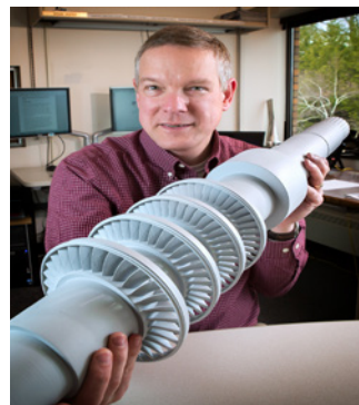
The high density of supercritical carbon dioxide enables order-of-magnitude smaller turbo machinery and components, reducing costs. (Image: General Electric)
