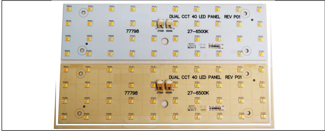
Figure 3-1. The control MULTI-WT1 LED module (top) and a second module (bottom) after 20,000 hrs of exposure to the 95°C elevated ambient temperature.
