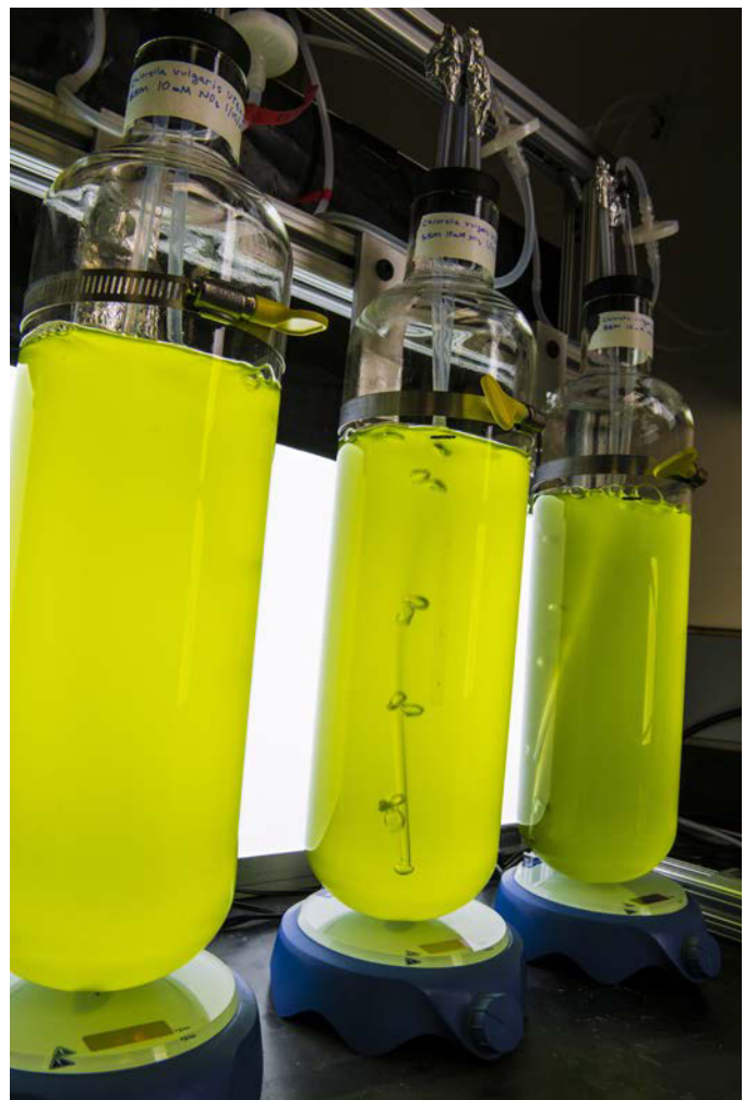
A chlorococcal strain of algae grows in a reactor in the Algal Lab in the Field Test Laboratory Building. Photo by Dennis Schroeder, NREL 55030
