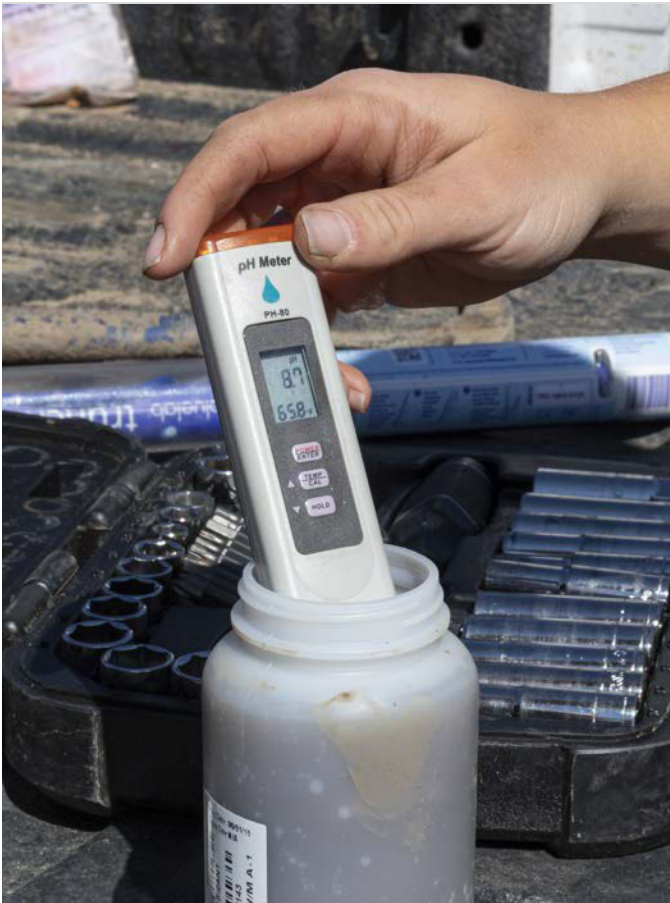
pH monitoring of groundwater from monitoring wells located north of the Field Test Laboratory Building at the STM site. Photo by Werner Slocum, NREL 56790
