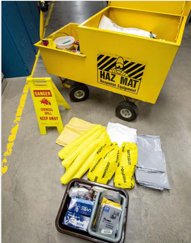
A hazardous waste spill cart located in an STM site laboratory, with various spill control materials displayed. Photo by Werner Slocum, NREL 56077
