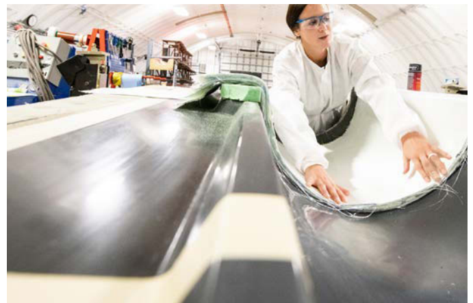
An NREL researcher applies fiberglass to a blade mold of a wind turbine at the NWTC. Photo by Dennis Schroeder, NREL 54066
