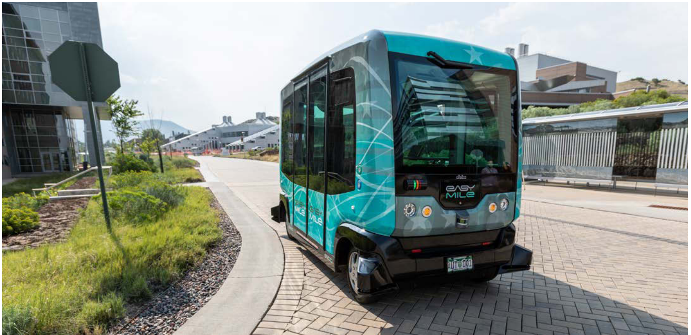
The EasyMile autonomous electric shuttle operated at the STM site during the 2018 Energy Innovation Trends - NREL Partner Forum. The shuttle, which is part of a planned NREL research project, can operate on fixed or on-demand routes, carrying up to 15 passengers. Photo by Werner Slocum, NREL 52563
