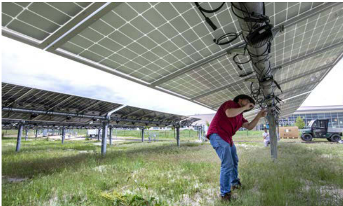
An NREL research technician runs cables to connect sensors and temperature probes to bifacial solar panels at the STM site. Bifacial panels can generate electricity from both the upper sky-facing and lower ground-facing sides of the panels. Photo by Werner Slocum, NREL 56760
