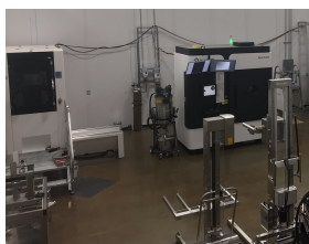
Figure 2. Arcam Spectra H installed at ORNL-Manufacturing Demonstration Facility
