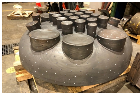
Figure 2. Forty-four percent scale A508 Cl1 Gr3 (1650 kg, 1270 mm) upper head with 27 penetrations, fabricated as one monolithic component (no welds)
