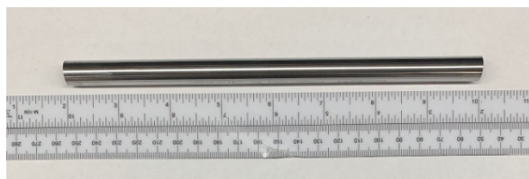
Figure 1: Photograph of free-standing ODS steel cladding tube produced by cold spray process.
