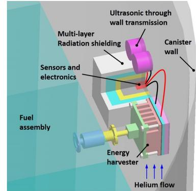
Energy harvester for powering sensing and communications.
