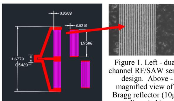
Figure 1. Left - dual-channel RF/SAW sensor design. Above - magnified view of a Bragg reflector (10µm line pitch).
