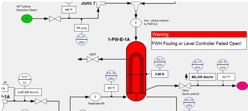
Prototypic Operator Interface for reporting of diagnostic findings.
