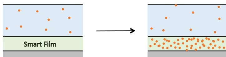
Figure 1. Schematic representation of “smart film chelating metal ions in solution.
