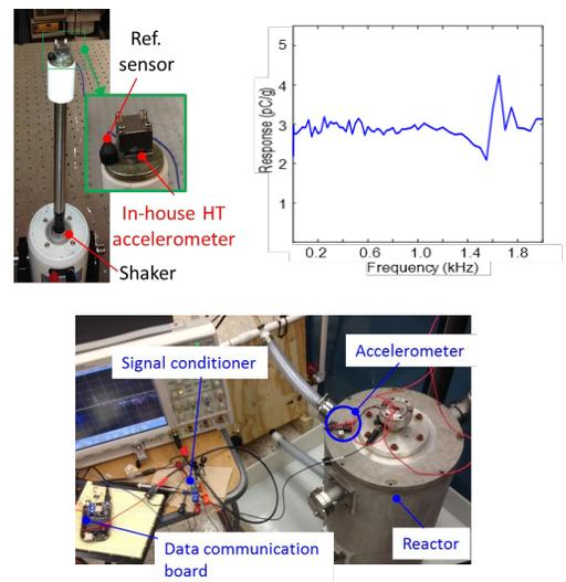
Figure 2. HT vibration sensor embedded in a miniaturized reactor with the wireless communication system.
