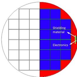
MCNP6 model to test the radiation shielding performance.
