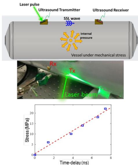
Figure 1. Laser stress sensing development.
