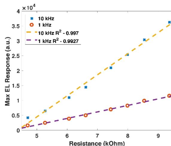
Figure 3. Maximum electroluminescent response of 3D printed ‘smart coating’ at various levels of resistance for two excitation features.
