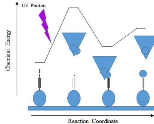
An asymmetric chemical potential between the SPM tip and surface-bound molecular tool (radical) will break an atomic bond at the tip apex, increasing the overall energy to a more thermodynamically favorable level than the initial condition.
